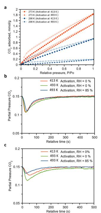
Fig. 4 (a)  $CO_2$  adsorption isotherms of Cu-1 at different temperatures as indicated after applying different degassing conditions and a pressure of 0.1 Pa. (b)  $CO_2$  breakthrough experiments at 273 K after applying different activation conditions as indicated; and (c)  $CO_2$  breakthrough experiments at 298 K after applying different activation conditions as indicated.
