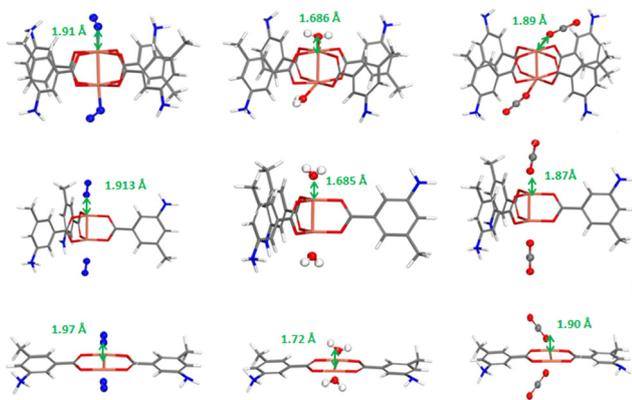
Fig. 7 The single CO<sub>2</sub>, N<sub>2</sub> and H<sub>2</sub>O adsorbed on the defective sites, at low loading.
