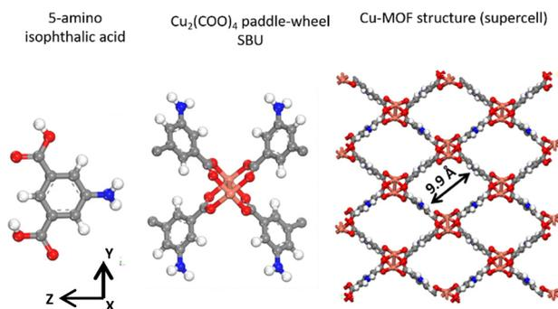
Fig. 1 Visualization of the monoclinic Cu(AIPA) structure represented as a  $4 \times 3 \times 2$  supercell (expanded along the  $x$ ,  $y$ , and  $z$  crystallographic axes) and viewed along the  $x$ -direction. The atomic color scheme is as follows: copper (Cu) – orange; carbon (C) – grey; oxygen (O) – red; nitrogen (N) – blue; hydrogen (H) – white.
