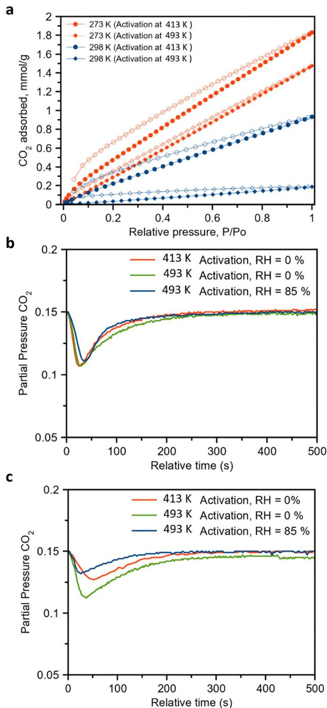
Fig. 4 (a) CO<sub>2</sub> adsorption isotherms of Cu-1 at different temperatures as indicated after applying different degassing conditions and a pressure of 0.1 Pa. (b) CO<sub>2</sub> breakthrough experiments at 273 K after applying different activation conditions as indicated; and (c) CO<sub>2</sub> breakthrough experiments at 298 K after applying different activation conditions as indicated.
