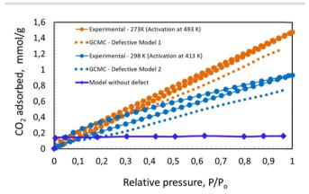
Fig. 6 Comparison between GCMC adsorption isotherms determined at different defects and the experimental CO2 adsorption isotherms of Cu-1 carried out at different degassing conditions. Defective model 1 corresponds to 30% of Tri-Cu(ı) and 65% of Tetra Cu(ıı) and 5% of Di-Cu(ı) and the defective model 2 corresponds to 35% of Tri-Cu(i) and 55% of tetra Cu(II) and 10% of Di-Cu(I)
