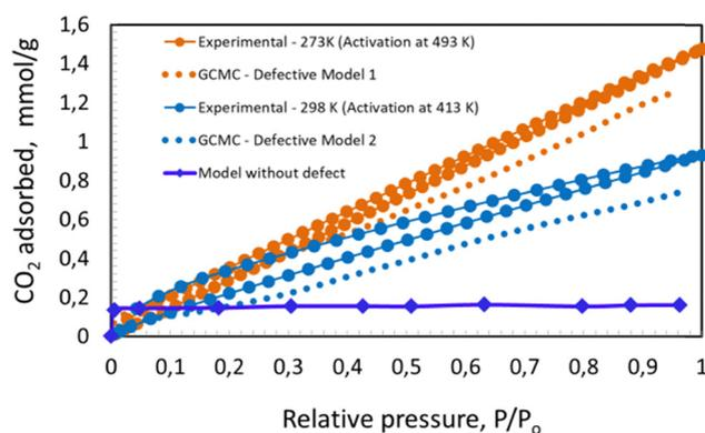
**Fig. 6** Comparison between GCMC adsorption isotherms determined at different defects and the experimental  $CO_2$  adsorption isotherms of Cu-1 carried out at different degassing conditions. Defective model 1 corresponds to 30% of Tri-Cu(I) and 65% of Tetra Cu(II) and 5% of Di-Cu(I) and the defective model 2 corresponds to 35% of Tri-Cu(I) and 55% of tetra Cu(II) and 10% of Di-Cu(I).
