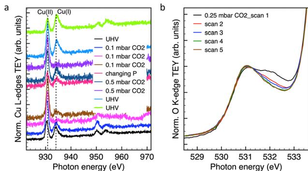
Fig. 5 NEXAFS spectra measured for Cu-1 under CO<sub>2</sub> pressure in the millibar range as indicated: (a) Cu L-edges (order of the experiments from bottom to top) and (b) O K edge.
