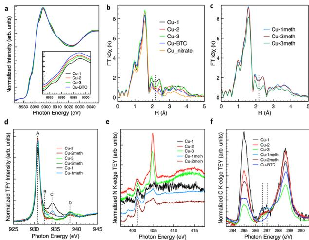
**Fig. 3** XANES (a) and FT-EXAFS spectra (b) of Cu-1, Cu-2 and Cu-3. Spectra are compared with experimental data of Cu-BTC and Cu nitrate (Sigma Aldrich). (c) Comparison of the FT-EXAFS spectra of samples Cu-1, Cu-2 and Cu-3 experimental spectra after washing with methanol. (d) Cu  $L_3$ -edge XAFS spectrum of samples as indicated. (e) N K-edge XAFS and (f) C K-edge XAFS. The spectra in the inset in (a) are y-axis shifted for a better visualization.
