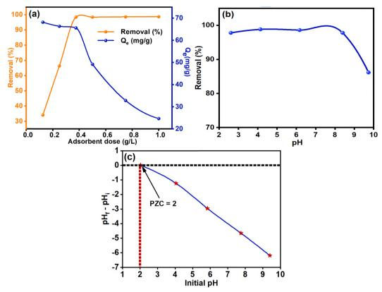
Fig. 5 (a) Effect of the PANi@DPC dosage on the OG decolorization performance (conditions: pH = 6.17; adsorption time = 2 h; OG concentration = 25 mg L<sup>-1</sup>; T = 25 °C), (b) evolution of OG dye removal performance as a function of pH (conditions: PANi@DPC dose = 0.375 g L<sup>-1</sup>; contact time = 2 h; OG concentration = 25 mg  $L^{-1}$ ; T = 25 °C) and (c) PZC determination of the PANi@DPC composite.
