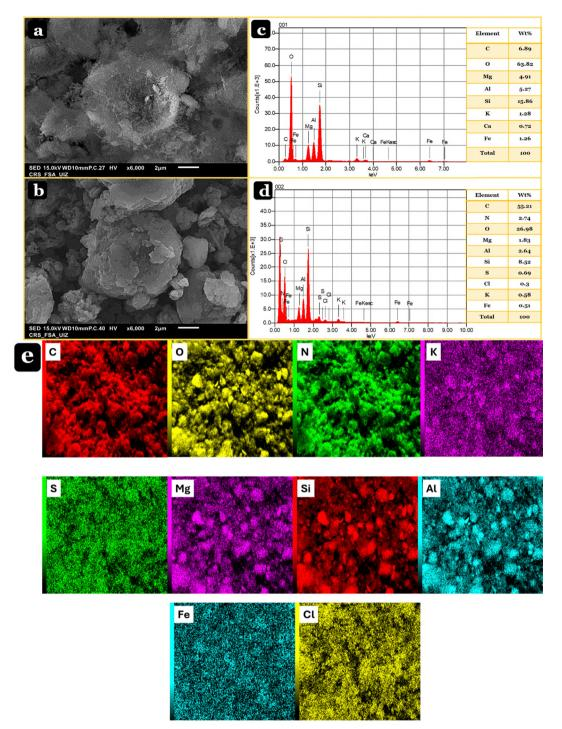
Fig. 3 SEM micrographs of (a) DPC and (b) the PANi@DPC composite and their respective EDS spectra (c) and (d) and (e) EDS elemental maps of the PANi@DPC composite.
