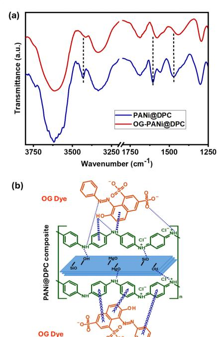
Fig. 10 (a) FTIR spectrum of PANi@DPC composite after OG dye adsorption, and (b) schematic representation of the proposed OG dye binding mechanism.
