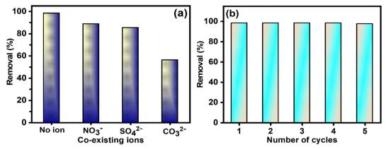
Fig. 11 (a) Influence of interfering ions on the OG dye decolorization by the PANi@DPC composite (pH = 6.17; equilibrium time = 2 h; adsorbent dose = 0.375 g  $L^{-1}$ ; 25 mg  $L^{-1}$  OG concentration; T = 298 K) and (b) OG dye removal yield for 5 times reuse of the PANi@DPC composite.
