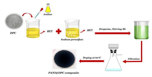
Fig. 1 Schematic diagram of the fabrication process of the PANi@DPC hybrid composite.
