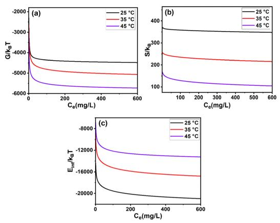
Fig. 9 Representations of (a) free enthalpy, (b) entropy and (c) internal energy functions for OG dye adsorption on the PANi@DPC composite.
