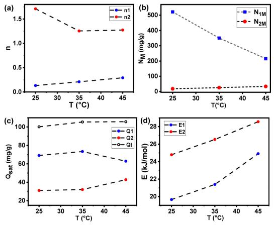
Fig. 8 Evolution of physicochemical parameters: (a) n, (b)  $N_{M}$ , (c)  $Q_{sat}$  and (d) E as a function of temperature for OG dye adsorption on the PANi@DPC hybrid composite.
