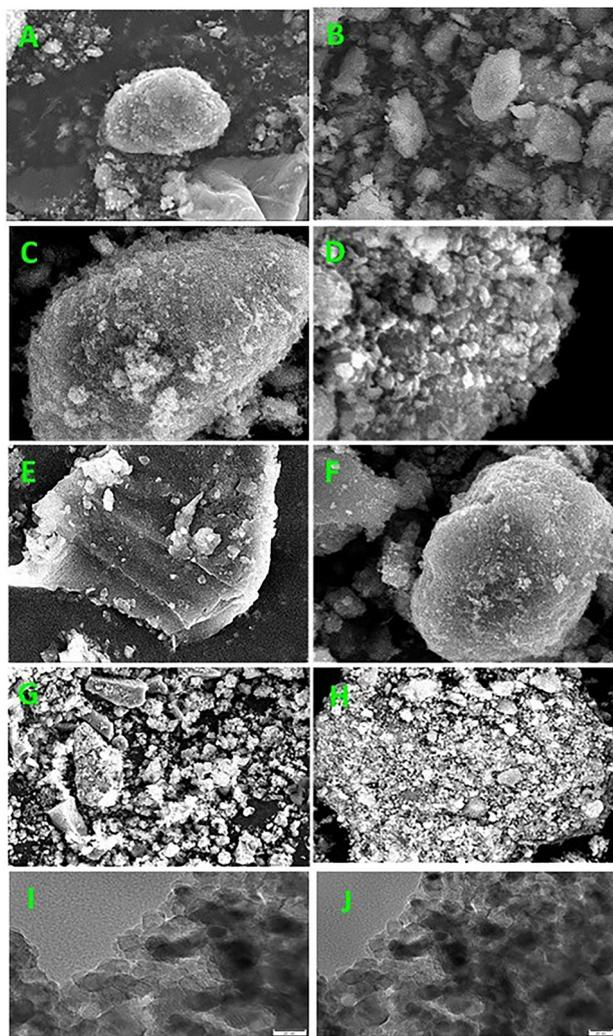
Fig. 2 SEM images of (A)  $\text{TiO}_2$  and (B) CP. Different molar composites: (C) 0.1, (D) 0.25, (E) 0.5, and (F) 1.0 M of  $\text{TiO}_2/\text{CP}$  (G)  $\text{Fe}^0\text{-TiO}_2$  and (H)  $\text{Fe}^0\text{-TiO}_2/\text{CP}$ , and (I) and (J) TEM of  $\text{TiO}_2$ .
