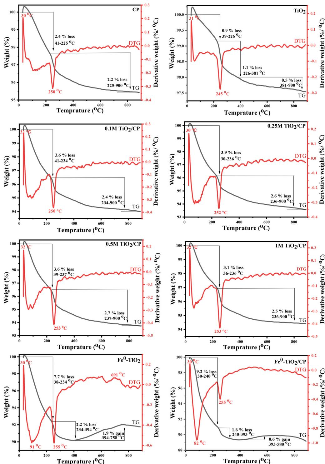
Fig. 3 TG/DTG profiles of pure CP, TiO<sub>2</sub>, 0.1, 0.25, 0.5, 1.0 M TiO<sub>2</sub>/CP, and Fe<sup>0</sup>-TiO<sub>2</sub> and Fe<sup>0</sup>-TiO<sub>2</sub>/CP composites measured at a heating rate of 10 K min<sup>-1</sup> under N<sub>2</sub> flow.
