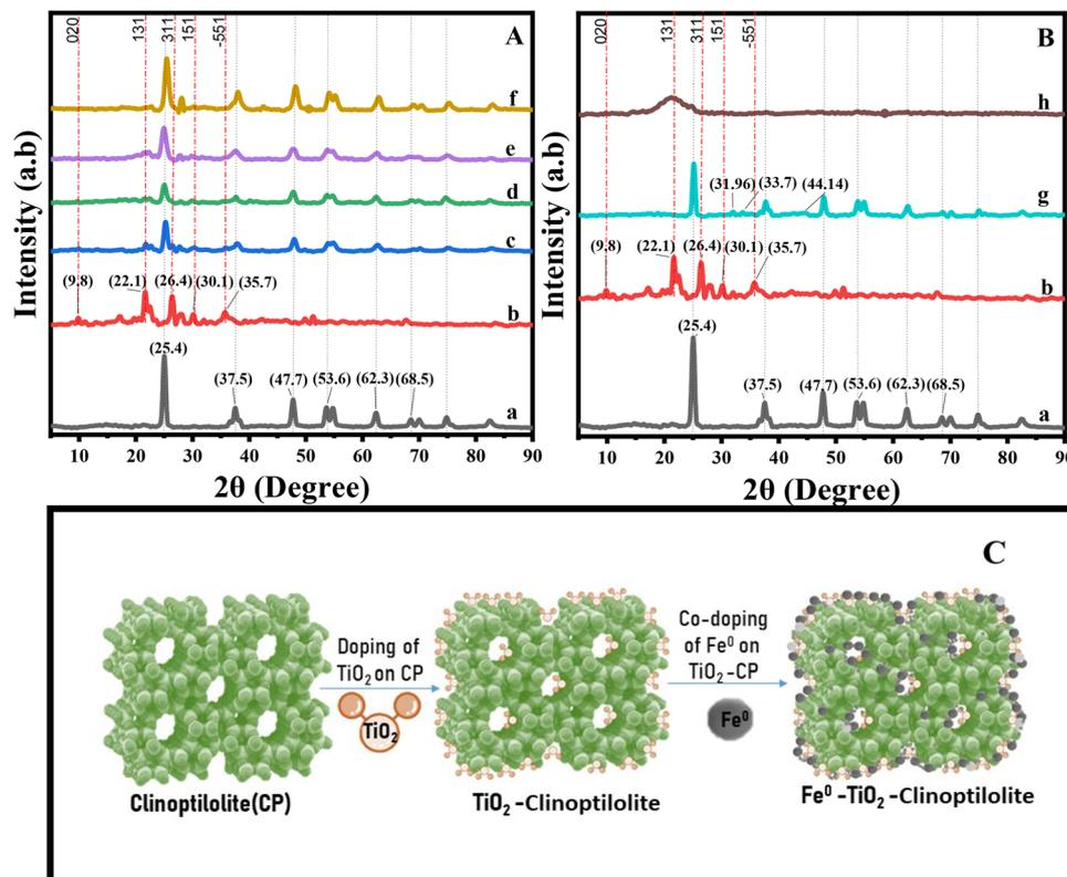
Fig. 1 XRD patterns of A: (a)  $\text{TiO}_2$ , (b) parent CP, (c) 0.1, (d) 0.25, (e) 0.5 and (f) 1.0 M  $\text{TiO}_2/\text{CP}$  and B: (g)  $\text{Fe}^0\text{-TiO}_2$  and (h)  $\text{Fe}^0\text{-TiO}_2/\text{CP}$ . C: doping and co-doping of  $\text{TiO}_2$  and  $\text{Fe}^0$ , respectively, on CP.
