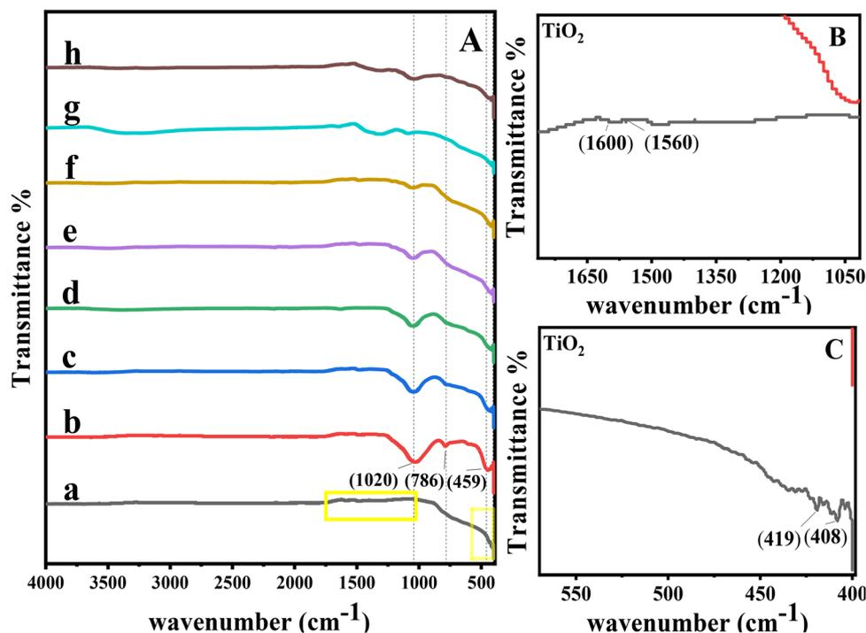
Fig. 4 FTIR spectra of A: (a) TiO<sub>2</sub>, (b) parent CP, (c) 0.1, (d) 0.25, (e) 0.5, (f) 1.0 M TiO<sub>2</sub>/CP, (g) Fe<sup>0</sup>-TiO<sub>2</sub>/CP and (h) Fe<sup>0</sup>-TiO<sub>2</sub>. B and C are the insets of A.
