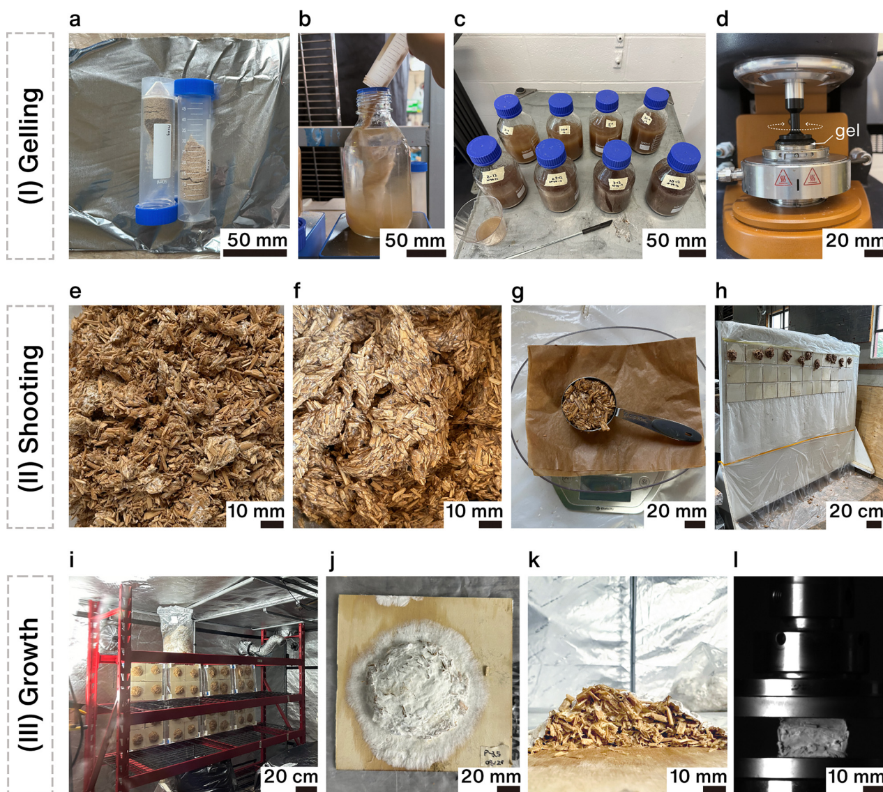
Fig. 3 Summary of mixture processing steps and experimental test set-ups from material preparation to final mycelium incubation: (a) autoclaving preparation of psyllium husk powder. (b) Stirring psyllium husk powder in distilled water. (c) Retention of psyllium husk gels for specific durations. (d) Rheometer with parallel plate geometry. (e) Original hemp–mycelium mixtures (five days after inoculation) with loose properties. (f) Mixing hemp–mycelium mixtures (five days after inoculation) with psyllium husk gel. (g) Extracting a single shooting sample from the mixing bowl and weighing it. (h) Shooting the sample onto the vertical surface. (i) Mycelium incubation in a vertical orientation. (j) and (k) Mycelium growth observation on the surface and across the cross-section. (l) Compression testing.
