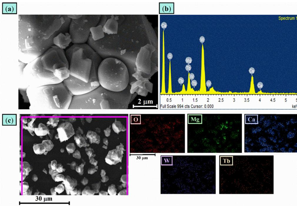
Fig. 6 (a) SEM image. (b) EDAX spectra. (c) Elemental mapping for the CMW:xTb<sup>3+</sup> (x = 6 mol%) phosphor.
