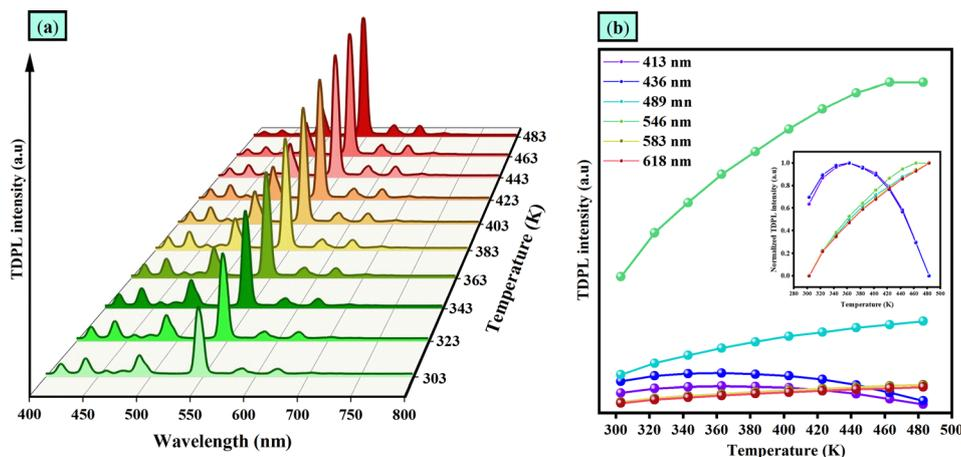
Fig. 8 (a) TDPL spectra for the CMW: $x\text{Tb}^{3+}$  ( $x = 6$  mol%) phosphors for  $\lambda_{\text{ex}} = 247$  nm. (b) Variation in TDPL intensity for the characteristic  $\text{Tb}^{3+}$  peaks with normalized TDPL intensity as shown in the inset.
