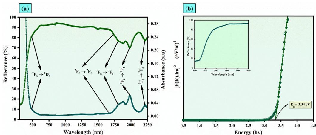
Fig. 7 (a) UV-vis-NIR spectra of the CMW:xTb<sup>3+</sup> (x = 6 mol%) phosphor. (b) Optical band gap calculation for the CMW:xTb<sup>3+</sup> (x = 6 mol%) phosphor using Tauc plot, with the variation in reflectance shown in the inset.
