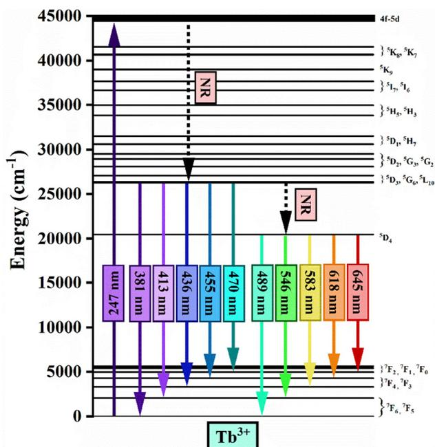
Fig. 2 Energy level of the Tb<sup>3+</sup> ion in the CMW:Tb<sup>3+</sup> phosphors.
