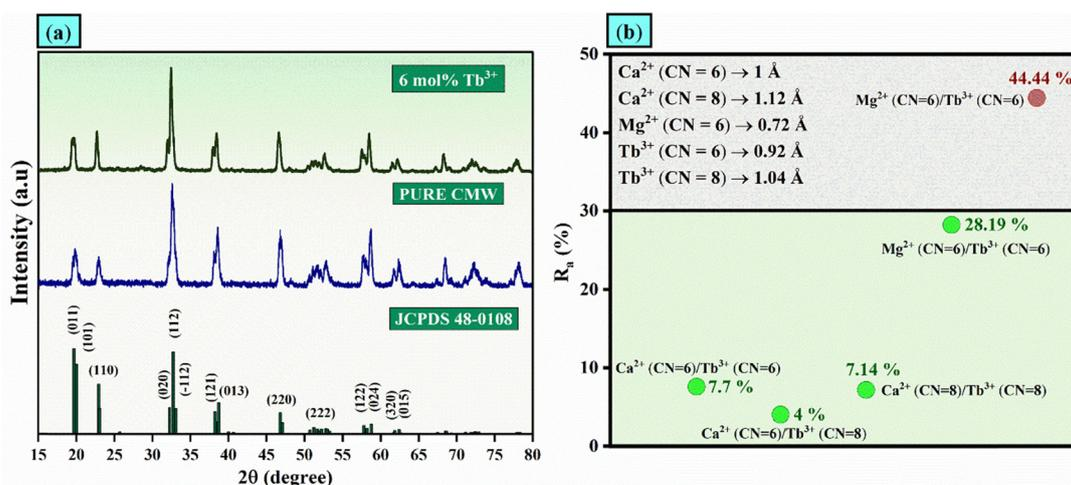
Fig. 4 (a) XRD patterns of CMW and optimized CMW: 6 mol% Tb<sup>3+</sup> phosphors in comparison with JCPDS file #48-0108. (b) Acceptable percentage difference in the radius for Ca<sup>2+</sup>/Tb<sup>3+</sup> and Mg<sup>2+</sup>/Tb<sup>3+</sup> pairs.
