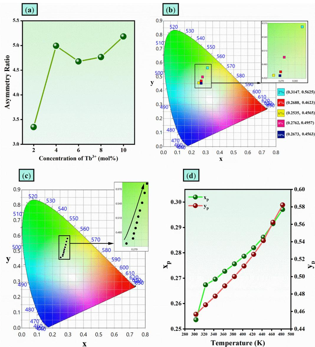
Fig. 11 (a) Variation in asymmetric ratio with Tb<sup>3+</sup> concentration. (b) CIE-1931 chromaticity diagram for the synthesized phosphor samples. (c) and (d) Temperature-dependent CIE coordinates of the optimized phosphor and its variation with the temperature.
