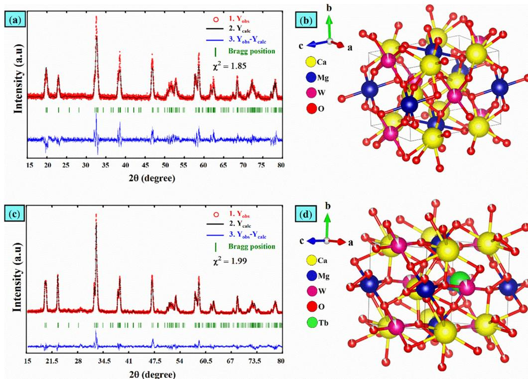
Fig. 5 (a) Results of the Rietveld refinement for CMW. (b) Unit cell of CMW drawn using the refined data. (c) Results of the Rietveld refinement for CMW:6 mol%  $\text{Tb}^{3+}$ . (d) Unit cell of CMW:6 mol%  $\text{Tb}^{3+}$  drawn using the refined data.
