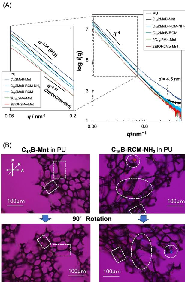
**Fig. 8** (A) SR-SAXS patterns of clay-loaded PU foams recorded in (left) small (0.06 <  $q$  < 0.2 nm<sup>-1</sup>) and (right) wide (0.06 <  $q$  < 3.0 nm<sup>-1</sup>) angle ranges. (B) Typical photographs under crossed polarizers for C<sub>16</sub>2MeB-Mnt and C<sub>16</sub>2MeB-RCM-NH<sub>3</sub>. The dotted circles and squares indicate dispersion in a thinner cell and aggregates in the cell wall, respectively.
