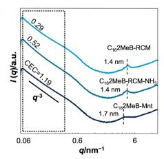
Fig. 9 SAXS patterns of mixtures of the premix solution with  $C_{16}2$ MeB-modified montmorillonite samples prepared using different layer charge densities.
