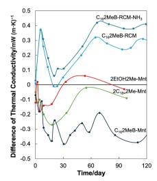
Fig. 7 Time-course profiles of the difference in the thermal conductivity  $(\Delta k)$  of polyurethane (PU) foam  $(k_{\rm wof})$  and organically modified montmorillonite-loaded PU foam  $(k_{\rm f})$ .
