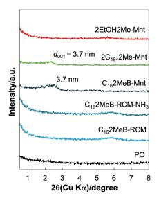
Fig. 5 Powder XRD patterns of the PO mixtures with organically modified montmorillonites.
