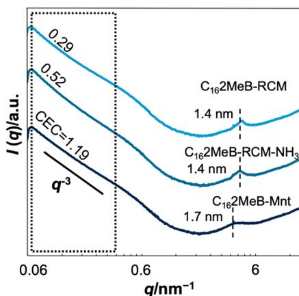
Fig. 9 SAXS patterns of mixtures of the premix solution with C<sub>16</sub>2MeB-modified montmorillonite samples prepared using different layer charge densities.
