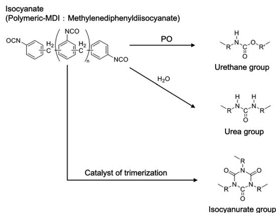
Fig. 1 Polymerization process of the urethane/urea/isocyanurate copolymer.
