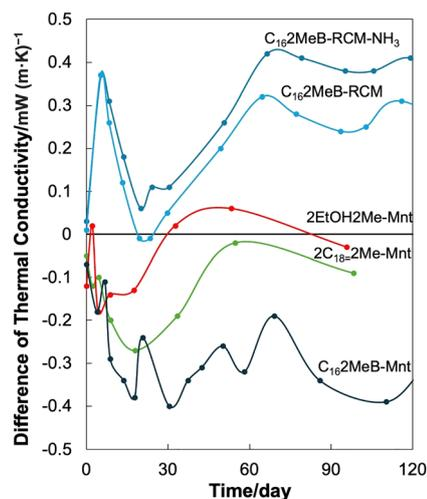
Fig. 7 Time-course profiles of the difference in the thermal conductivity ( $\Delta k$ ) of polyurethane (PU) foam ( $k_{\text{wof}}$ ) and organically modified montmorillonite-loaded PU foam ( $k_{\text{f}}$ ).
