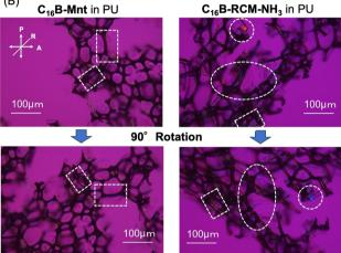
Fig. 8 (A) SR-SAXS patterns of clay-loaded PU foams recorded in (left) small  $(0.06 < q < 0.2 \text{ nm}^{-1})$  and (right) wide  $(0.06 < q < 3.0 \text{ nm}^{-1})$  angle ranges. (B) Typical photographs under crossed polarizers for C<sub>16</sub>2MeB-Mnt and C<sub>16</sub>2MeB-RCM-NH<sub>3</sub>. The dotted circles and squares indicate dispersion in a thinner cell and aggregates in the cell wall, respectively.
