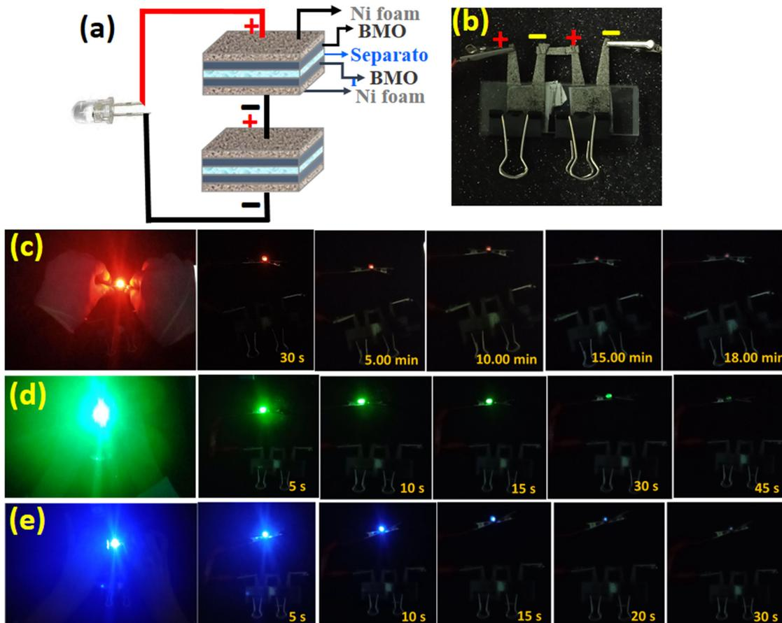
Fig. 9 (a) and (b) Schematic and photographic images of the series connection of two symmetric supercapacities and (c) and (e) real-time feasibility of the supercapacerty tested by energizing red, green, and blue LEDs.
