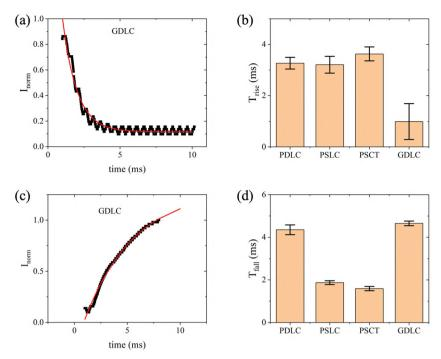
Fig. 7 Response time analysis: (a) response raise time calculated from transmission measurements using GDLC as an example. (b) Bar chart comparing  $\tau_{\rm rise}$  value across four materials. (c) Response fall time calculated from transmission measurements using GDLC as an example. (d) Bar chart comparing  $\tau_{\text{fall}}$  value across the four different devices
