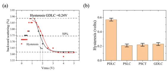
Fig. 5 (a) Schematic illustration on how the hysteresis was determined, presented for the GDLC sample. (b) Comparison of determined hysteresis values for all four types of devices.
