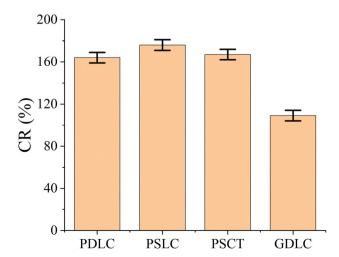
Contrast ratio comparing of the four smart glass device structures.
