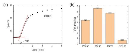
Fig. 6 (a) Schematic illustration of the determination of the threshold voltage using data obtained from the GDLC device. (b) Bar chart comparing the threshold voltage,  $V_{\text{th}}$ , for the four different devices.
