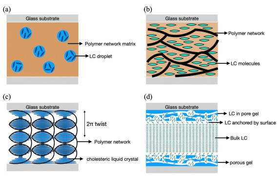
Fig. 1 Schematic illustration of (a) a polymer-dispersed liquid crystal device (PDLC), (b) a polymer-stabilised nematic device (PSLC), (c) a polymer-stabilised cholesteric texture (PSCT), and (d) a gel-glass dispersed liquid crystal (GDLC).
