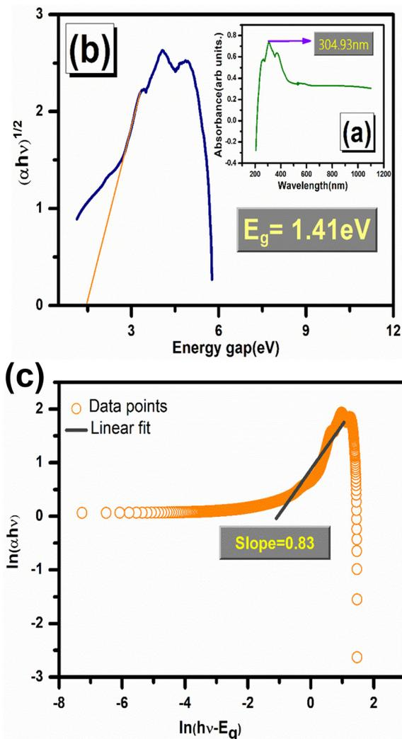
Fig. 3 (a) Absorbance spectrum [inset] and (b) Tauc plot of BiFeWO<sub>6</sub>. (c) Calculation of the  $n$  value from  $\ln(\alpha h\nu)$  versus  $\ln(h\nu - E_g)$  of BiFeWO<sub>6</sub>.
