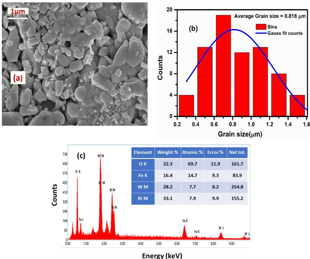
Fig. 2 (a) SEM micrograph, (b) Gaussian fitting grain size using ImageJ software, and (c) EDX spectrum confirming the presence of all constituent elements.
