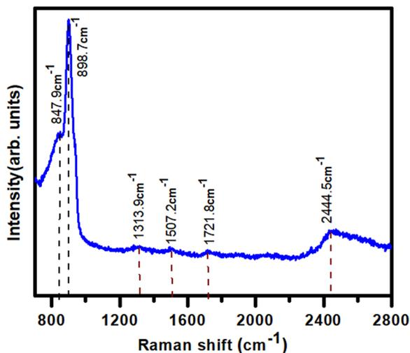
Fig. 4 Raman spectrum of BiFeWO<sub>6</sub>.
