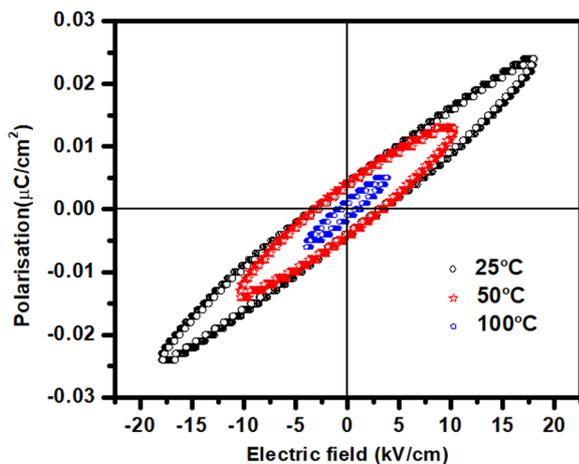
Fig. 10  $P$ - $E$  hysteresis loop of  $\text{BiFeWO}_6$ .
