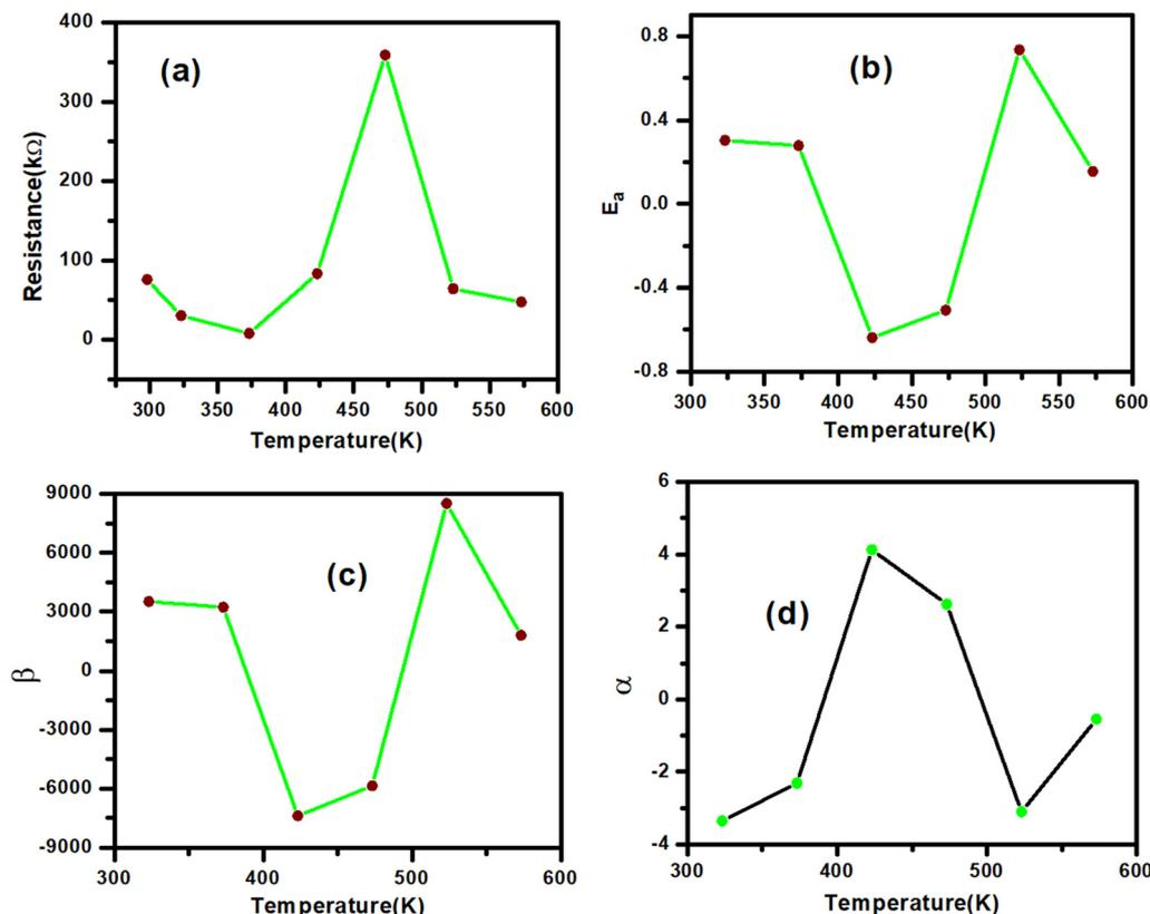
Fig. 9 (a) Variation in resistance with temperature, (b) activation energy versus temperature, (c) thermistor constant versus temperature and (d) sensitivity factor versus temperature of BiFeWO<sub>6</sub>.
