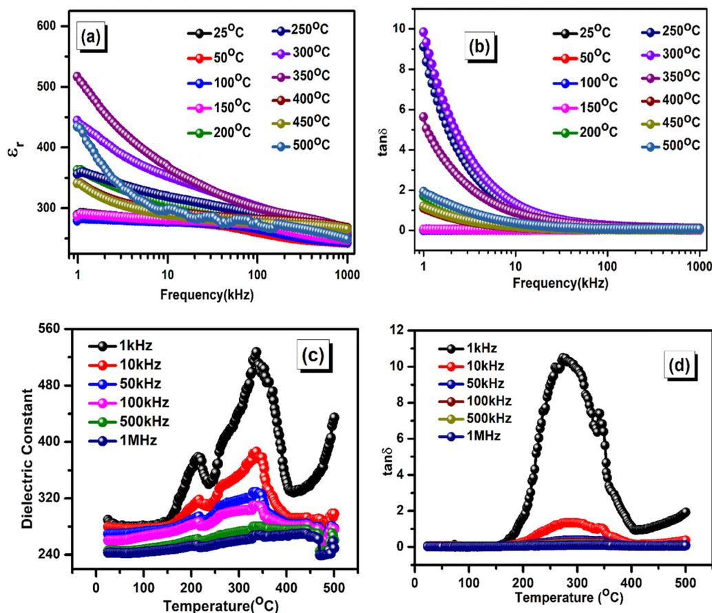
Fig. 5 (a) and (b) Variation of the dielectric constant and tangent loss versus frequency. (c) and (d) Variation of the dielectric constant and tangent loss versus temperature of BiFeWO<sub>6</sub>.
