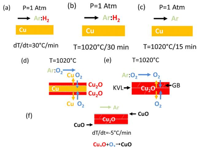
Fig. 2 Schematic representation of the process used for the growth of  $\text{Cu}_2\text{O}$  by thermal oxidation of Cu under Ar:  $\text{O}_2$  (a) temperature ramp (b) short reduction and anneal of Cu under Ar:  $\text{H}_2$  (c) purging of hydrogen (d) and (e) thermal oxidation and (f) controlled cool down.
