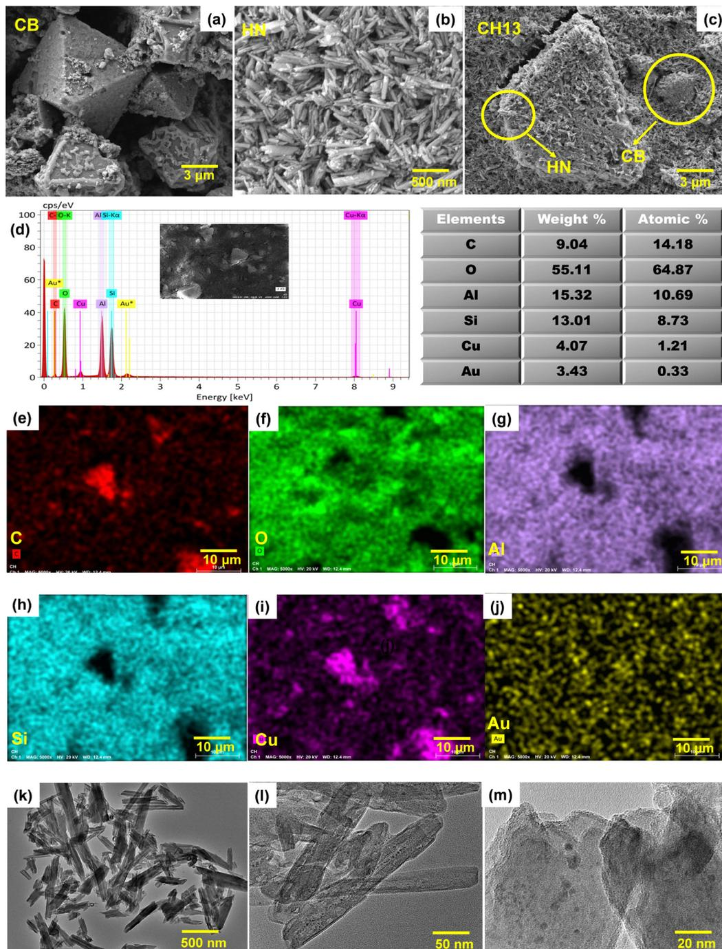
Fig. 3 FESEM images of (a) CB, (b) HN, and (c) CH13, (d) EDS spectrum of CH13, (e) and (j) elemental coloured mapping of various elements, and (k)–(m) HRTEM images of CH13 at different magnifications.
