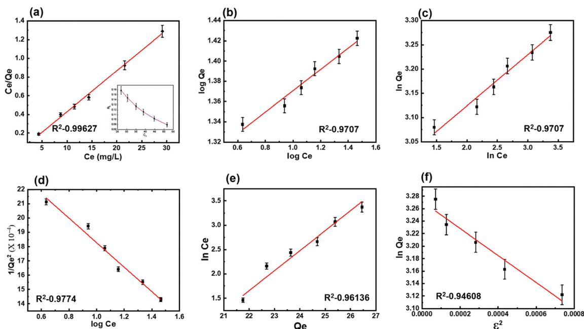
Fig. 5 Plots with linearly fitted adsorption isotherms for (a) Langmuir (inset RL plot), (b) Freundlich, (c) Halsey, (d) Harkins–Jura, (e) Temkin, and (f) D–R models.
