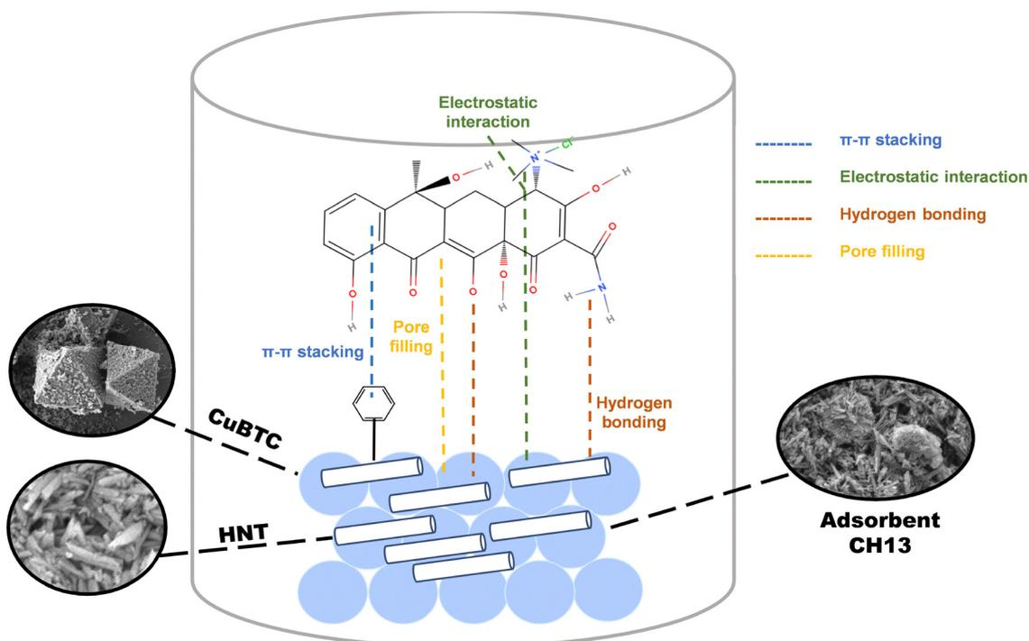
Scheme 2 Adsorption scheme of TC onto CH13.
