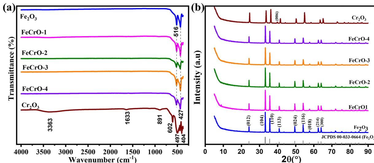
Fig. 3 (a) FTIR spectra; (b) XRD patterns of pristine  $\text{Fe}_2\text{O}_3$ ,  $\text{Cr}_2\text{O}_3$  and all the Cr-doped  $\text{Fe}_2\text{O}_3$  (FeCrO-1, FeCrO-2, FeCrO-3 and FeCrO-4).
