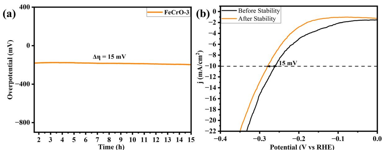
Fig. 9 (a) Chronopotentiometry of the best Cr-doped  $\text{Fe}_2\text{O}_3$  (FeCrO-3), and (b) its LSV polarization curves before and after chronopotentiometry.
