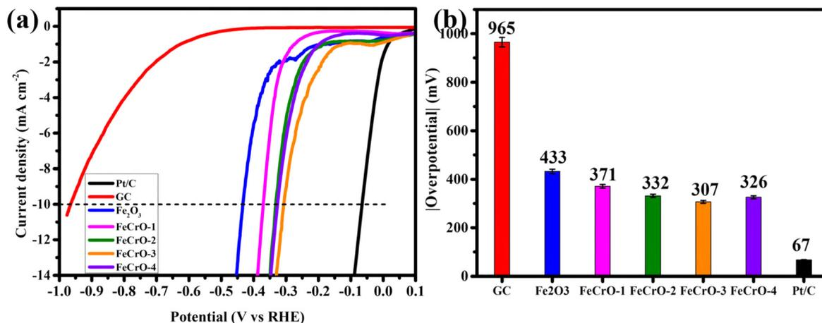
Fig. 6 Electrochemical performance for HER in alkaline medium (1 M KOH): (a) linear sweep voltammetry (LSV) curves at 10 mV s<sup>-1</sup> for Pt/C, GC, Fe<sub>2</sub>O<sub>3</sub>, and Cr-doped Fe<sub>2</sub>O<sub>3</sub> samples. (b) Overpotential values at 10 mA cm<sup>-2</sup> for the same materials. Error bars represent standard deviation from triplicate measurements.
