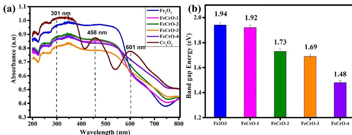
Fig. 5 (a) UV-visible spectra, and (b) energy bandgap of Fe<sub>2</sub>O<sub>3</sub>, Cr<sub>2</sub>O<sub>3</sub> and all the Cr-doped Fe<sub>2</sub>O<sub>3</sub> (FeCrO-1, FeCrO-2, FeCrO-3 and FeCrO-4).
