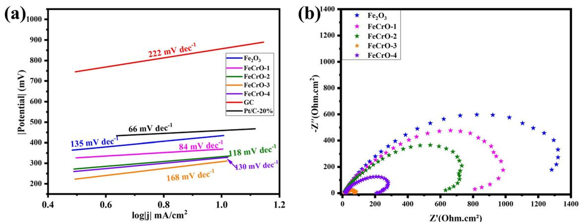
Fig. 7 (a) Tafel plots and (b) EIS Nyquist plots for Fe<sub>2</sub>O<sub>3</sub>, and Cr-doped Fe<sub>2</sub>O<sub>3</sub> samples.
