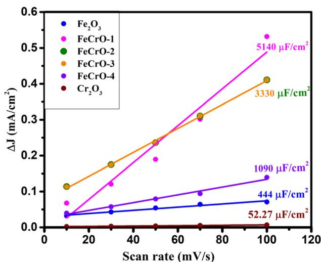
Fig. 8 Scan rate dependence of the current densities at 0.05 V of pristine  $\text{Fe}_2\text{O}_3$ ,  $\text{Cr}_2\text{O}_3$  and all the Cr-doped  $\text{Fe}_2\text{O}_3$  (FeCrO-1, FeCrO-2, FeCrO-3 and FeCrO-4).
