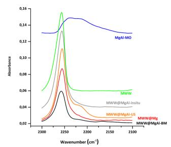
Fig. 8 FT-IR spectra of the different MWW@samples at maximum coverage of CDCl<sub>3</sub> at 298 K and 90 mbar.
