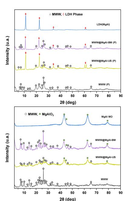
Fig. 5 XRD patterns of multi-component MWW@LDH materials obtained following synthesis method (III): (top) as-synthesized samples; (bottom) calcined samples.
