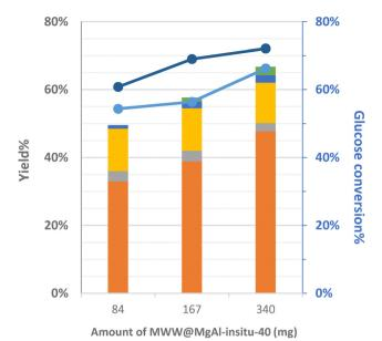
Fig. 14 Catalytic results for the oxidation of glucose varying the MWW@MgAl-in situ-40 loading. Reaction conditions: glucose (0.96 mmol), catalyst (0.066 g mixed oxide phase), 20% H<sub>2</sub>O<sub>2</sub> (5.76 mmol), dioxane (4.75 mL). ■ Erythrose yield%, ■ glycoaldehyde dimer yield%, ■ arabinose yield%, ■ fructose yield%, ■ FA yield%, • glucose conversion%.
