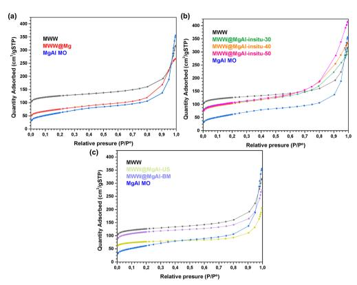
Fig. 3 N<sub>2</sub> adsorption isotherms. (a) Multi-component MWW@Mg materials obtained through method (I). (b) Multi-component MWW@MgAl-in situ materials obtained through method (II) with different LDH contents. (c) Multi-component MWW@LDH materials obtained following synthesis method (III).
