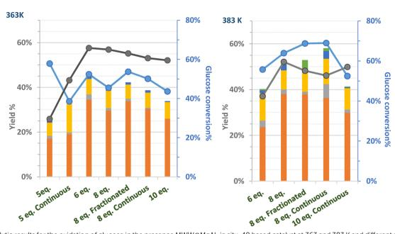
Fig. 12 Catalytic results for the oxidation of glucose in the presence MWW@MgAl-in situ-40 based catalyst at 363 and 383 K and different addition mode and ratio H<sub>2</sub>O<sub>2</sub>/glucose. Reaction conditions: glucose (0.96 mmol), catalyst (0.066 g mixed oxide phase), dioxane (4.75 mL). Erythrose yield%, ■ glycolaldehyde dimer yield%, ■ arabinose yield%, ■ fructose yield%, ■ FA yield%, ● glucose conversion%, ● FA selectivity%.
