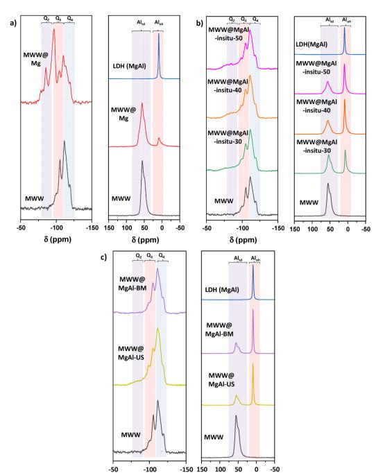
Fig. 2 <sup>29</sup>Si BD MAS NMR (left) and <sup>27</sup>Al MAS NMR (right) spectra. (a) As-synthesized multi-component MWW@Mg materials obtained through method (I). (b) As-synthesized multi-component MWW@MgAl-in situ materials obtained following synthesis method (II) with different LDH content. (c) As-synthesized multicomponent MWW@LDH materials obtained following synthesis method (III) using ultrasonic and ball milling techniques.
