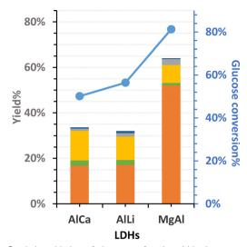
Fig. 9 Catalytic oxidation of glucose to formic acid in the presence LDH based catalysts. Reaction conditions: glucose (0.96 mmol), catalyst (0.15 g), EtOH (4.75 mL), 20% H<sub>2</sub>O<sub>2</sub> (5.76 mmol), 363 K, 5 h. ■ erythrose yield%, ■ glycolaldehyde dimer yield%, ■ arabinose yield%, ■ fructose yield%, ■ FA yield%, • glucose conversion%
