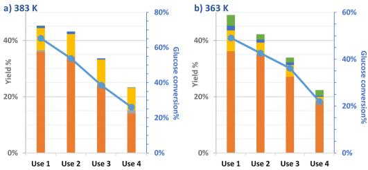
Fig. 15 Study of MWW@MgAl-in situ-40 recycling for the catalytic oxidation of glucose to formic acid catalyst at 383 K (a) and 363 K (b) and 8 equivalents of  $H_2O_2$ . Reaction conditions: glucose (0.96 mmol), catalyst (0.066 g mixed oxide phase), dioxane (4.75 mL).  $\blacksquare$  Erythrose yield%,  $\blacksquare$  qlycoaldehyde dimer yield%,  $\blacksquare$  arabinose yield%,  $\blacksquare$  fructose yield%,  $\blacksquare$  fluctose conversion%.
