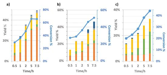
Fig. 10 Catalytic oxidation of glucose to formic acid in the presence LDH derived based catalysts, (a) Mg/Al MO, (b) MWW@MgAl-in situ-40 and (c) MWW@MgAlCe-in situ-40. ■ Erythrose yield%, ■ glycolaldehyde dimer yield%, ■ arabinose yield%, ■ fructose yield%, ■ FA yield%, ■ glucose conversion%. Reaction conditions: glucose (0.96 mmol), catalyst (0.066 g mixed oxide phase), EtOH, (4.75 mL), 30% H<sub>2</sub>O<sub>2</sub> (5.76 mmol), 363 K.
