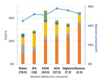
Fig. 11 Catalytic results for the oxidation of glucose to FA in the presence MWW@MgAl-in situ-40 catalyst in different solvents. Reaction conditions: glucose (0.96 mmol), catalyst (0.066 g mixed oxide phase), solvent, (4.75 mL), 20%  $H_2O_2$  (5.76 mmol), 363 K, 7.5 h.  $\blacksquare$  erythrose yield%,  $\blacksquare$  glycolaldehyde dimer yield%,  $\blacksquare$  arabinose yield%,  $\blacksquare$  fructose yield%,  $\blacksquare$  FA yield%,  $\blacksquare$  glucose conversion%.
