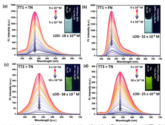
Fig. 4 Change in emission spectra (10  $\mu$ M in 1,4-dioxane) by gradual addition of TN and FN: (a) TT1 + TN ( $\lambda_{ex}$  = 310 nm), (b) TT1 + FN ( $\lambda_{ex}$  = 310 nm), (c) TT2 + TN ( $\lambda_{ex}$  = 430 nm), and (d) TT3 + TN ( $\lambda_{ex}$  = 430 nm), respectively; inset pictures correspond to the emission before and after pesticide addition under 365 nm UV light.
