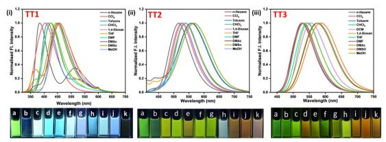
Fig. 2 The solvatochromic features of the compounds (i) TT1, (ii) TT2 and (iii) TT3; the solvents (a) hexane, (b) carbon tetrachloride (CCl<sub>4</sub>), (c) toluene, (d) dichloromethane (DCM), (e) chloroform (CHCl<sub>3</sub>), (f) 1,4-dioxane, (g) tetrahydrofuran (THF), (h) N,N-dimethylformamide (DMF), (i) dimethylsulphoxide (DMSO), (j) dimethylacetamide (DMAc), and (k) MeOH.
