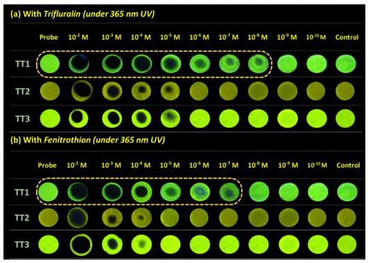
Fig. 7 TT1@WP (10 μM) was assessed before and after exposure to (a) TN and (b) FN with gradually diluted concentrations (under a 365 nm UV lamp).
