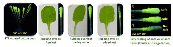
Fig. 9 TT1-coated fluorescent cotton buds as a handy on-site pesticide detector.
