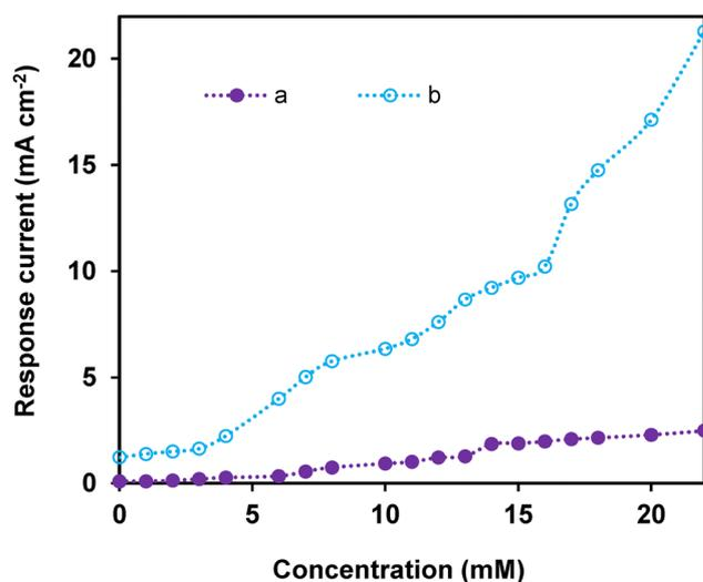
Fig. 10 The variation of response current for graphite coated ANCC (a) and ANCC/Ag–ZnO nanocomposite (b) electrodes with the change in AA concentration in phosphate buffered 5.0 mM  $[\text{Fe}(\text{CN})_6]^{3/4-}$  solution. Conditions: scan rate,  $100 \text{ mV s}^{-1}$ ; potential,  $-0.2$  to  $+0.6 \text{ V}$ , pH 7.0.
