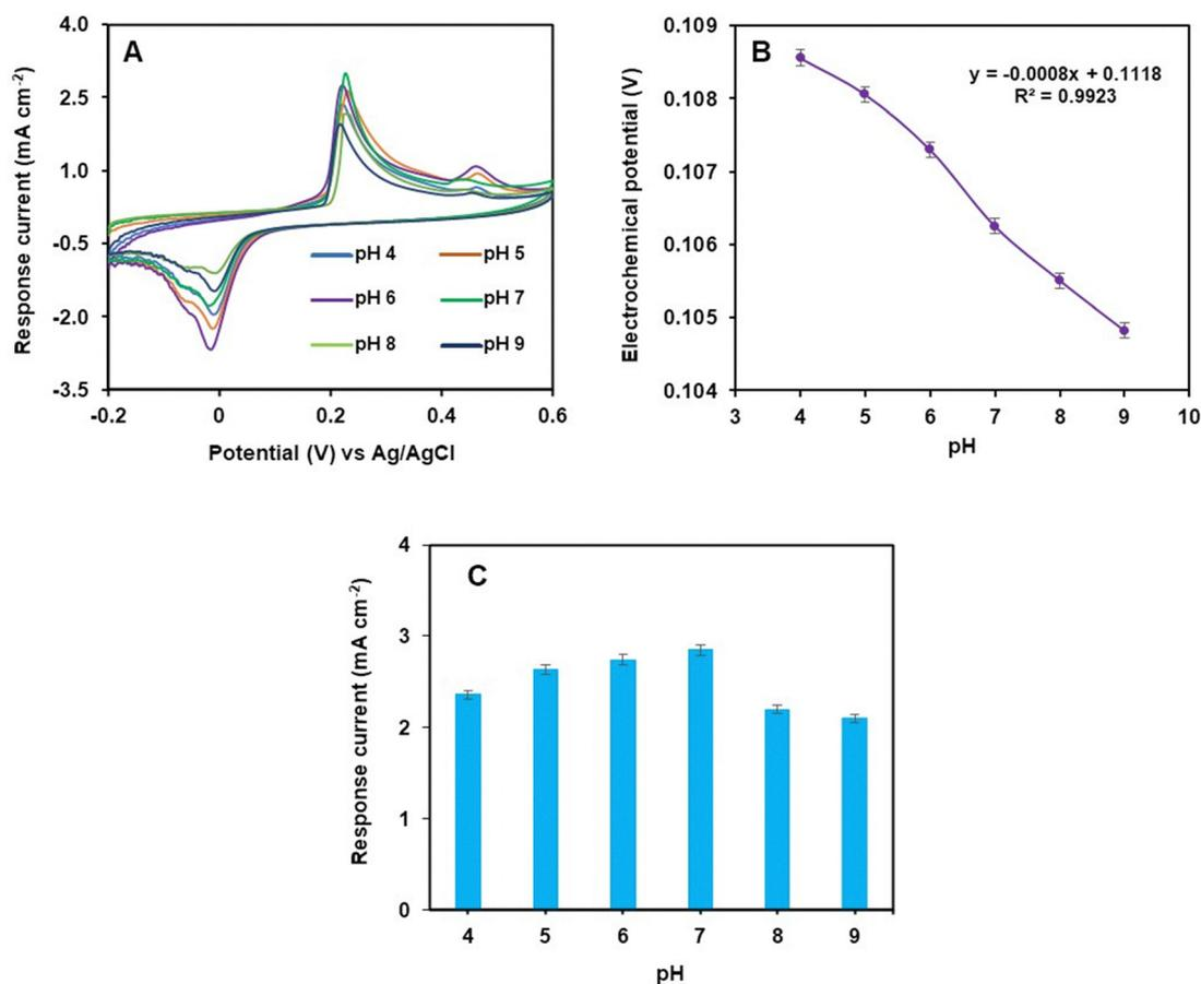
Fig. 9 (A) CV curves of the graphite coated ANCC/Ag-ZnO nanocomposite electrode in phosphate buffered 5.0 mM  $[\text{Fe}(\text{CN})_6]^{3/4-}$  solution (pH variable) containing 4.0 mM AA at a scan rate of  $100 \text{ mV s}^{-1}$ . (B) Electrochemical potential,  $E_{1/2}$  versus pH curve and (C) pH tuning in a bar diagram.
