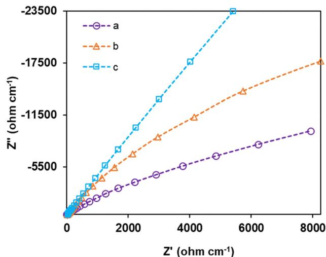
Fig. 8 The Nyquist plots of the EIS of graphite coated ANCC (a), Ag-ZnO (b) and ANCC/Ag-ZnO nanocomposite (c) electrodes in phosphate buffered (pH 7.0) 5.0 mM  $[\text{Fe}(\text{CN})_6]^{3/4-}$  solution over the frequency range of  $5 \times 10^{-2}$  to  $5 \times 10^{-5}$  Hz measured at a  $100 \text{ mV s}^{-1}$  scan rate.
