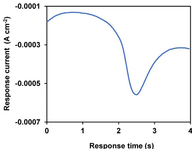
Fig. 14 Response time profile of the graphite coated ANCC/Ag-ZnO nanocomposite electrode upon exposure to phosphate buffered solution (pH 7.0) containing 4.0 mM AA. Conditions: scan rate 100 mV s<sup>-1</sup>.
