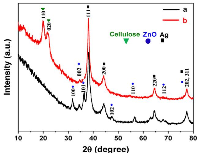
Fig. 5 X-ray diffraction (XRD) patterns of powder deposits obtained from the hybrid Ag-ZnO (a) and ANCC/Ag-ZnO nanocomposite (b) particles at a continuous scan rate of  $10^\circ \text{ min}^{-1}$ . Conditions: Cu  $K\alpha$  radiation ( $\lambda \gg$ ), 1.5406 Å; tube voltage, 33 kV; tube current, 45 mA.
