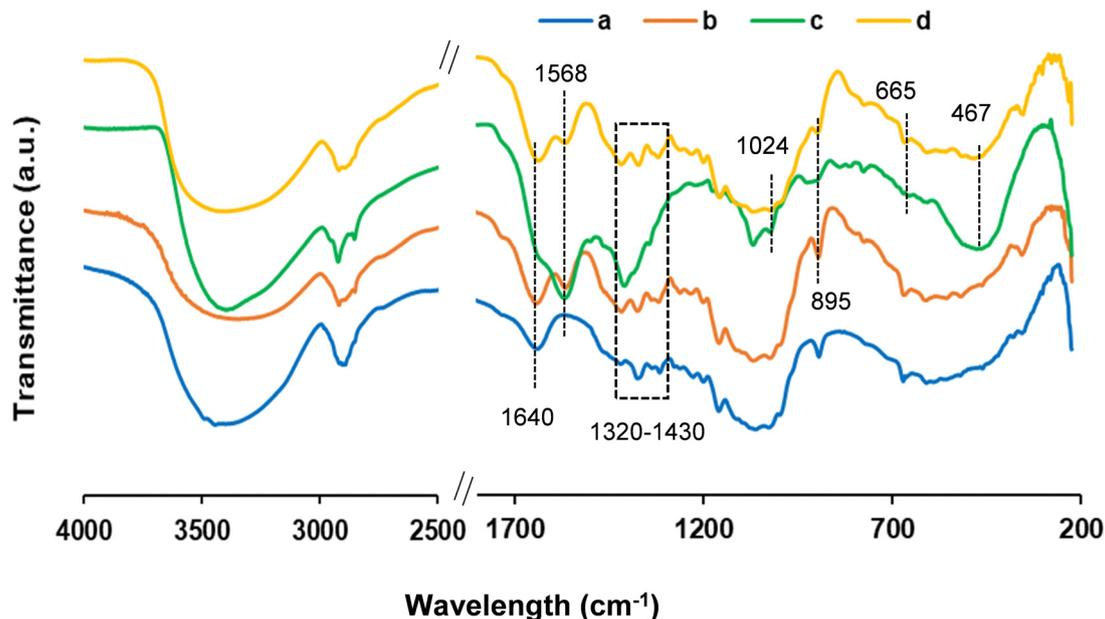
Fig. 2 FTIR spectra of NCC particles (a), ANCC particles (b), the Ag-ZnO hybrid (c) and ANCC/Ag-ZnO nanocomposite (d) particles taken in KBr pellets.
