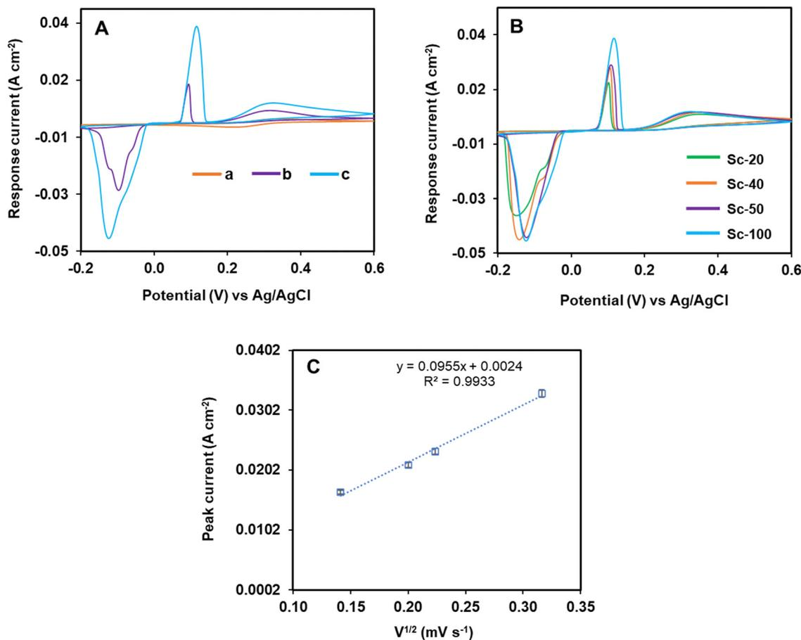
Fig. 6 (A) CV curves of the respective graphite coated ANCC (a), hybrid Ag-ZnO (b) and ANCC/Ag-ZnO nanocomposite (c) electrode in phosphate buffered (pH 7.0) 5.0 mM  $[\text{Fe}(\text{CN})_6]^{3/4-}$  solution at a scan rate of  $100 \text{ mV s}^{-1}$ . (B) Scan rate effect on CV curves of the graphite coated ANCC/Ag-ZnO nanocomposite electrode in phosphate buffered (pH 7.0) 5.0 mM  $[\text{Fe}(\text{CN})_6]^{3/4-}$  solution. (C) A plot of peak current versus the square root of the scan rate.
