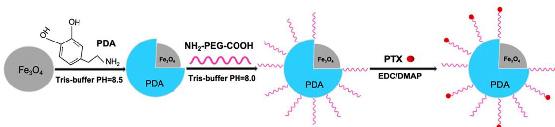
Fig. 1 Schematic representation of the synthesis of Fe<sub>3</sub>O<sub>4</sub>@PDA-PEG-PTX NPs.
