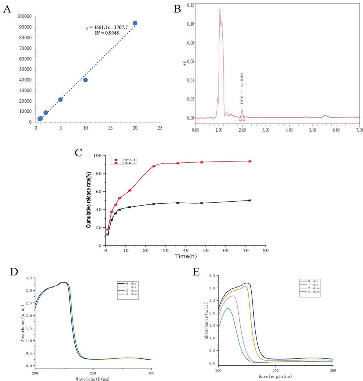
**Fig. 3** (A) Standard curve for HPLC of PTX. (B) HPLC of Fe<sub>3</sub>O<sub>4</sub>@PDA-PEG-PTX NPs. (C) PTX release from Fe<sub>3</sub>O<sub>4</sub>@PDA-PEG NPs at different pH values over 72 h. (D) UV-Vis spectrogram of the nanomaterials at PH = 7.4. (E) UV-Vis spectrogram of the nanomaterials at pH = 5.5.
