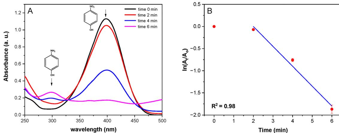
Fig. 8 (A) UV-vis absorption spectra and (B) pseudo-first-order kinetic profile for the catalytic hydrogenation of 4-nitrophenol (4-NP) to 4-aminophenol (4-AP) mediated by  $NaBH_4$  as the reducing agent and CuO/poly(DVB) as the catalyst. Experimental conditions: 0.1 mM 4-NP, 0.5 mM  $NaBH_4$ , and 20 mg CuO/poly(DVB).
