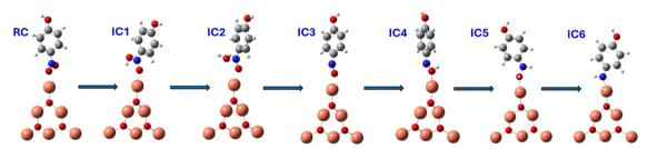
Fig. 9 Reaction pathway for the hydrogenation of nitrophenol to aminophenol catalyzed by CuO nanoparticles, as investigated through density functional theory (DFT) calculations.
