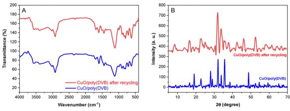
Fig. 12 (A) FTIR spectra and (B) XRD patterns of the CuO/poly(DVB) catalyst before and after four catalytic recycling cycles.
