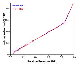
Fig. 7 N<sub>2</sub> adsorption/desorption isotherm of CuO/poly(DVB).
