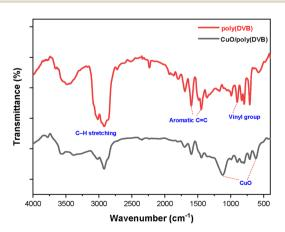
Fig. 2 FTIR spectra of poly(DVB) and CuO/poly(DVB)
