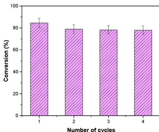
Fig. 11 Recycling experiments for the catalytic reduction of 4-NP to 4-AP. Reaction conditions: [4-NP] = 0.1 mM, [NaBH<sub>4</sub>] = 10 mM, weight of CuO/poly(DVB) is 20 mg.
