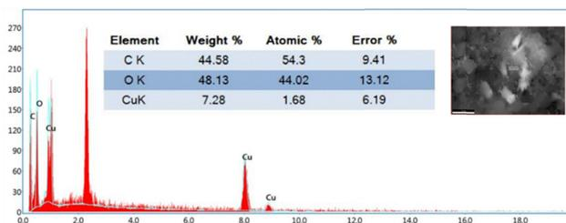
Fig. 6 Energy dispersive X-ray spectroscopy (EDS) of CuO/poly(DVB).
