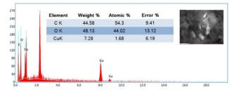
Fig. 6 Energy dispersive X-ray spectroscopy (EDS) of CuO/poly(DVB)
