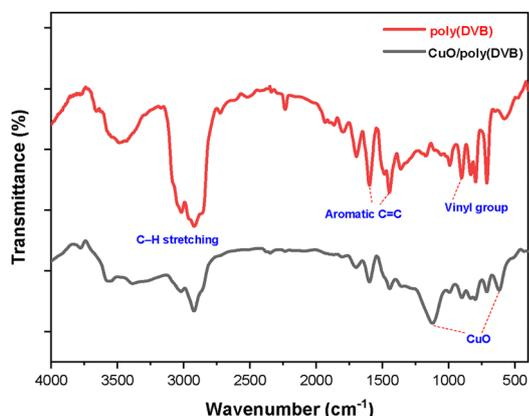
**Fig. 2** FTIR spectra of poly(DVB) and CuO/poly(DVB).
