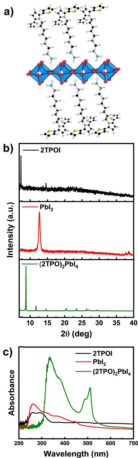
Fig. 3 (a) Schematic of the perovskite structure with 2TPO ligands coordinated with lead iodide octahedra. (b) XRD data and (c) UV-Vis absorbance spectra for  $(2\text{TPO})_2\text{PbI}_4$  thin film and both of its precursor compounds, showing the distinct behavior of the new perovskite composition.
