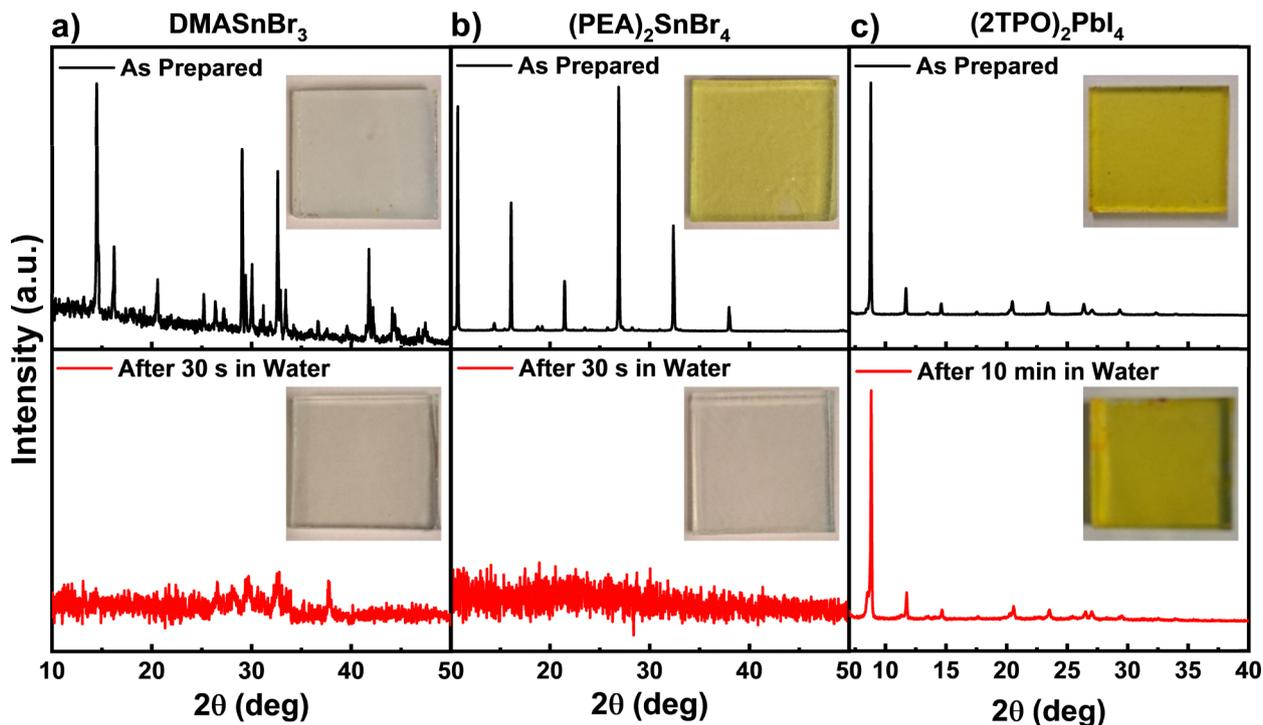
Fig. 2 Water stability of thin film forms of (a)  $\text{DMASnBr}_3$ , (b)  $(\text{PEA})_2\text{SnBr}_4$ , and (c)  $(2\text{TPO})_2\text{PbI}_4$  perovskites. (a)–(c) XRD data for the thin films as prepared (black) and after immersion in water (red) for either 30 s or 10 min. Insets show corresponding photographs of the thin film samples on a glass substrate.
