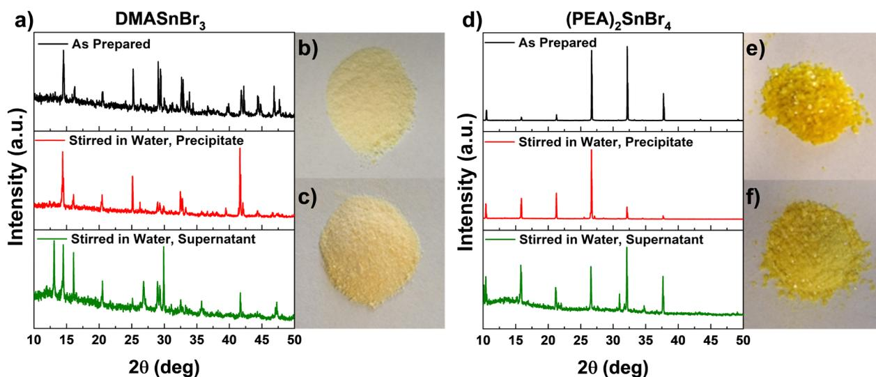
Fig. 1 Water stability of microcrystalline powder forms of (a)–(c)  $\text{DMASnBr}_3$  and (d)–(f)  $(\text{PEA})_2\text{SnBr}_4$  perovskites. (a) and (d) XRD data for the powders as prepared (black) and after 2 h of stirring in water then settling and decanting, with analysis of the precipitate (red) and the dried supernatant (green). Photographs are also shown of the powders (b) and (e) as prepared and (c) and (f) as precipitate after 2 h stirred in water.
