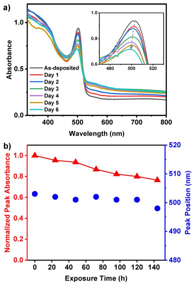
Fig. 6 (a) UV-Vis absorbance spectra for the  $(2\text{TPO})_2\text{PbI}_4$  thin film during continuous exposure to air of 85% relative humidity at room temperature, with an inset showing a zoomed-in view of the absorbance peak. (b) The absorbance peak normalized to the peak value for the as-deposited film (left axis, red) and the wavelength peak position (right axis, blue) vs. exposure time to 85% relative humidity.
