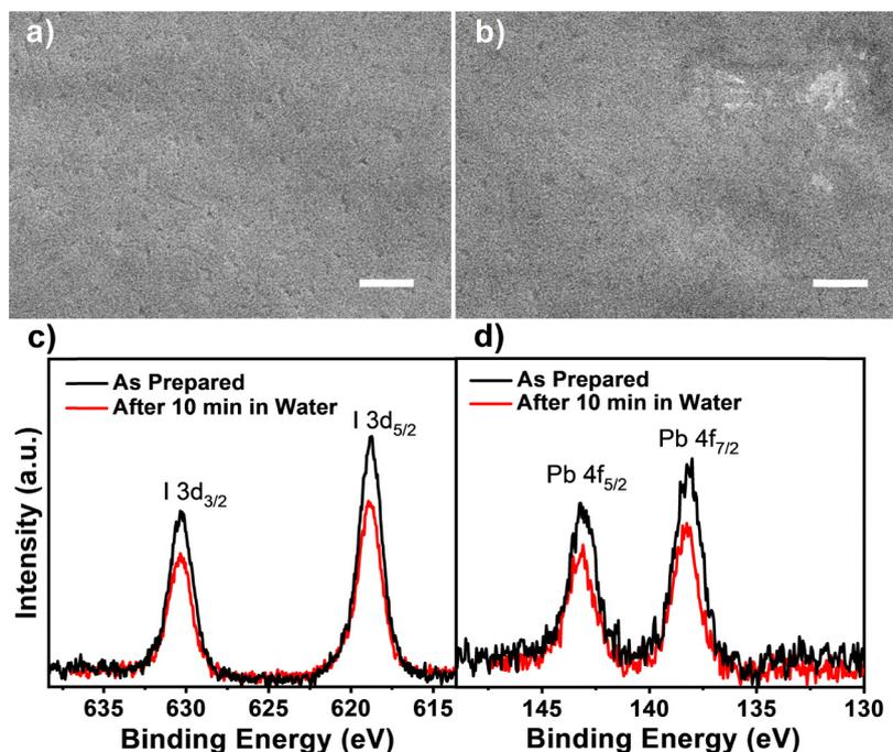
Fig. 7 SEM images of a  $(2\text{TPO})_2\text{PbI}_4$  thin film (a) before and (b) after 10 min immersed in water. The scale bar is 1  $\mu\text{m}$  in both. XPS spectra of the (c) I 3d and (d) Pb 4f regions for thin films of  $(2\text{TPO})_2\text{PbI}_4$  perovskite before (black) and after 10 min immersed in water (red).
