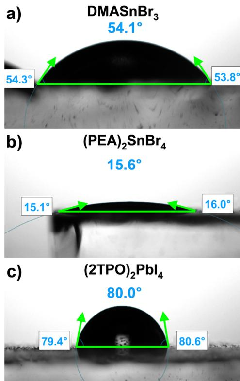
Fig. 4 Contact angle measurements for water droplets on thin films of (a)  $\text{DMASnBr}_3$ , (b)  $(\text{PEA})_2\text{SnBr}_4$ , and (c)  $(2\text{TPO})_2\text{PbI}_4$ . The angle shown above the droplet is the average of measurements from both sides of the droplet image.
