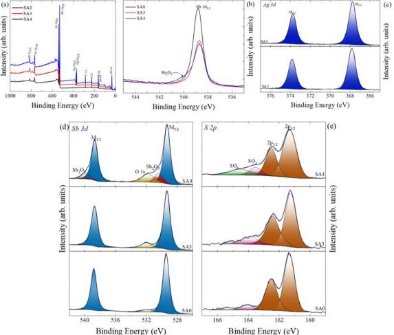
(a) and (b) XPS survey spectra, (c)-(e) core spectra of Ag 3d, Sb 3d, and S 2p of the silver-doped antimony sulfide film.
