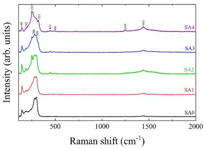
Fig. 2 Raman spectra of silver-doped antimony sulfide thin films.
