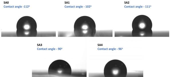
Fig. 5 Contact angle of silver-doped antimony sulfide thin films.
