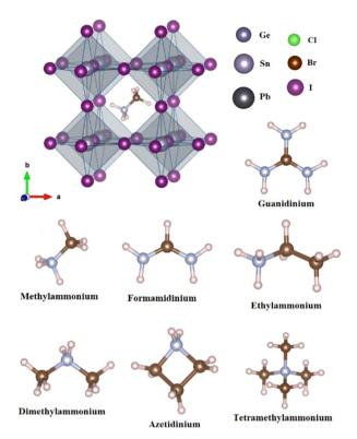
**Fig. 1** Schematic illustration of ABX<sub>3</sub>. In this representation, carbon, nitrogen, and hydrogen atoms are depicted using dark brown, gray, and light pink colors, respectively. Reproduced with permission.<sup>35</sup> Copyright 2023, MDPI.
