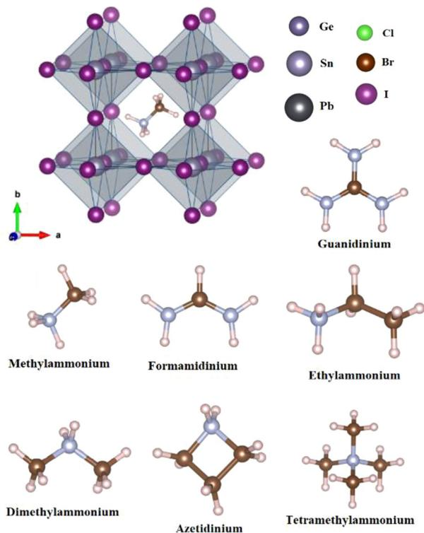
Fig. 1 Schematic illustration of  $ABX_3$ . In this representation, carbon, nitrogen, and hydrogen atoms are depicted using dark brown, gray, and light pink colors, respectively. Reproduced with permission.<sup>35</sup> Copyright 2023, MDPI.
