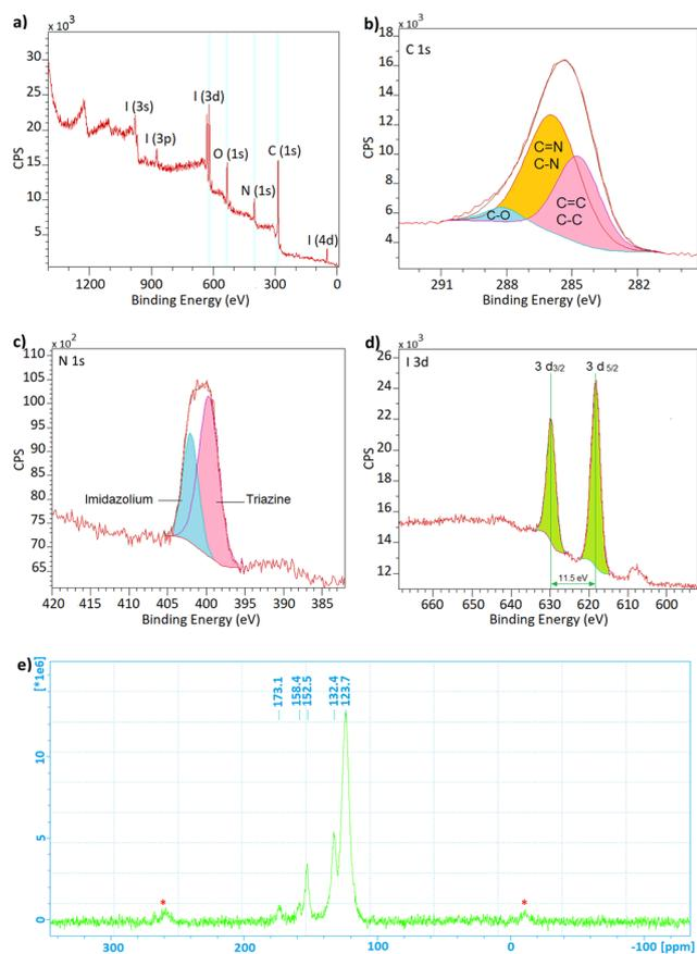
Fig. 3 XPS spectrum of I-CTF-1: (a) survey, (b) C 1s, (c) N 1s, and (d) I 3d. (e)  $^{13}C$  CP-MAS NMR spectrum of I-CTF-1 (the peaks marked by red stars are the spinning resonance of the aromatic rings).
