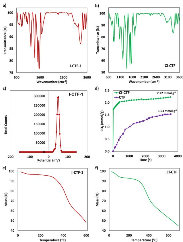
Fig. 2 FTIR spectra for (a) I-CTF-1 and (b) Cl-CTF. (c) Zeta potential curve for I-CTF-1. (d)  $\text{CO}_2$  adsorption capacity (1 bar  $\text{CO}_2$  at room temperature) for Cl-CTF and CTF (CTF without imidazolium units). TG pattern for (e) I-CTF-1 and (f) Cl-CTF.
