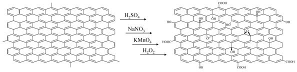
Fig. 1 Schematic of graphene oxide synthesis from graphene
