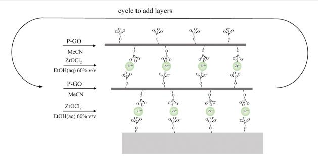
Fig. 4 Idealized reaction schematic of Phosphate-terminated silica surface with Zr<sup>4+</sup> followed by exposure to P-GO. Two P-GO deposition cycles are shown
