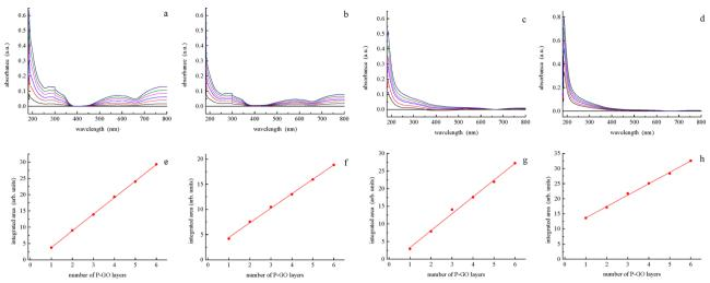
Fig. 7 Absorbance data and integrated areas P-GO layers bound through Zr<sup>4+</sup> complexation (2 min reaction time, (a) and (e)); P-GO layers bound through Zr<sup>4+</sup> complexation (4 min reaction time, (b) and (f)), P-GO layers with BP1 interlayer spacers (c) and (g), and P-GO layers with BP2 interlayer spacers (d) and (h).
