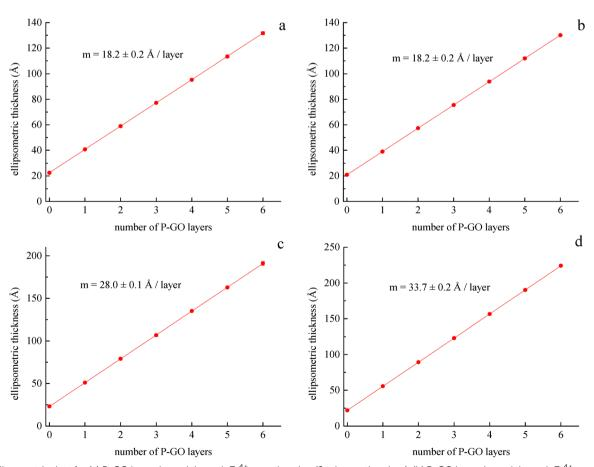
Fig. 6 Ellipsometric data for (a) P-GO layers bound through  $Zr^{4+}$  complexation (2 min reaction time), (b) P-GO layers bound through  $Zr^{4+}$  complexation (4 min reaction time), (c) P-GO layers with BP1 interlayer spacers, and (d) P-GO layers with BP2 interlayer spacers. The data reported are the average of 3 samples with typical uncertainties of 0.1-0.2 Å.
