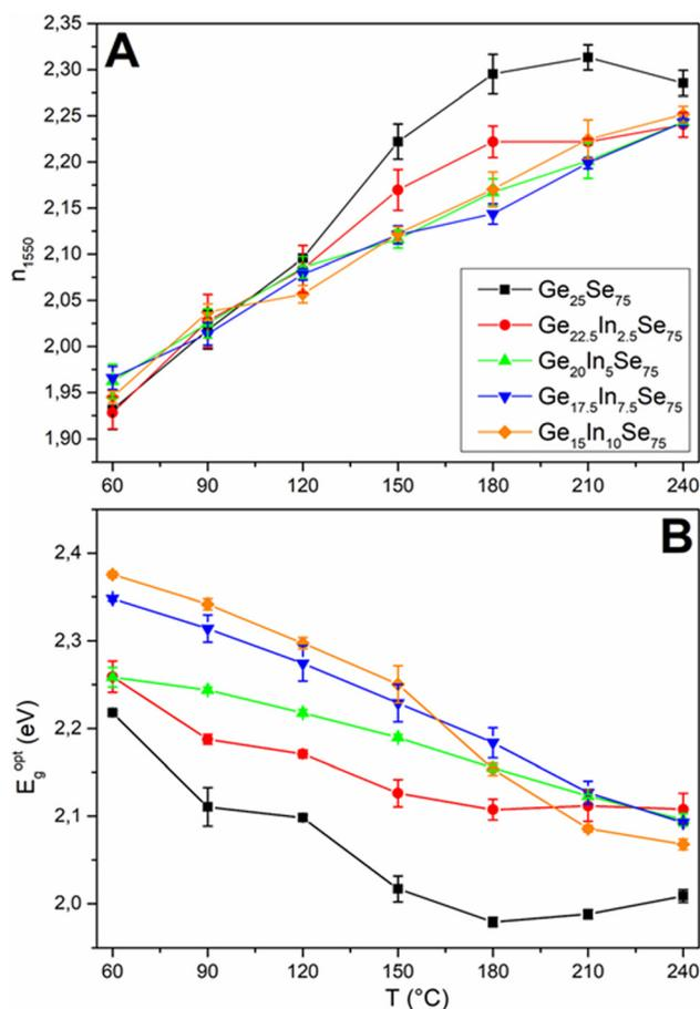
Fig. 4 The refractive index at 1550 nm  $n_{1550}$  (A) optical bandgap  $E_g^{\text{opt}}$  (B) of  $\text{Ge}_{25-x}\text{In}_x\text{Se}_{75}$  ( $x = 0, 2.5, 5, 7.5$  and  $10$ ) thin films in dependence on hard-baking temperature.
