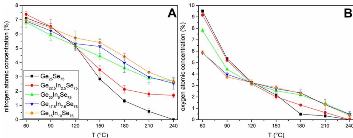
Fig. 3 The total nitrogen (A) and oxygen (B) content (as obtained from EDX analysis) in  $\text{Ge}_{25-x}\text{In}_x\text{Se}_{75}$  ( $x = 0, 2.5, 5, 7.5$  and  $10$ ) thin films representing organic residuals in dependence on hard-baking temperature.
