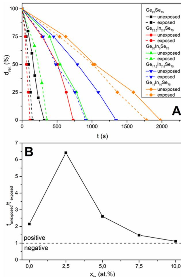
Fig. 8 The etching curves (A) and etching rates ratios (B) of  $\text{Ge}_{25-x}\text{In}_x\text{Se}_{75}$  ( $x = 0, 2.5, 5, 7.5$  and  $10$ ) thin films annealed at  $210\text{ }^\circ\text{C}$  before and after  $532\text{ nm}$  exposure.
