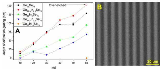
Fig. 9 The depths of diffraction gratings fabricated in  $\text{Ge}_{25-x}\text{In}_x\text{Se}_{75}$  ( $x = 0, 2.5, 5, 7.5$  and  $10$ ) thin films annealed at  $210^\circ\text{C}$  (A) along with the SEM scan of a representative diffraction grating (B). No diffraction gratings were produced in  $\text{Ge}_{15}\text{In}_{10}\text{Se}_{75}$  thin films.
