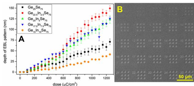
Fig. 10 The depths of EBL patterned  $\text{Ge}_{25-x}\text{In}_x\text{Se}_{75}$  ( $x = 0, 2.5, 5, 7.5$ , and  $10$ ) thin films annealed at  $210^\circ\text{C}$  in dependence on electron exposure dose (A) together with the SEM scan of a typical EBL pattern (B).
