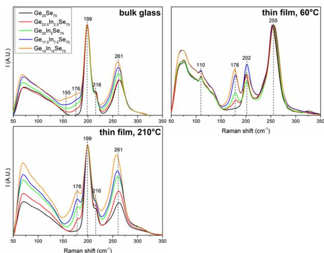
Fig. 6 The Raman spectra of  $\text{Ge}_{25-x}\text{In}_x\text{Se}_{75}$  ( $x = 0, 2.5, 5, 7.5$ , and  $10$ ) source bulk glasses together with the spectra of as-prepared thin films ( $60^\circ\text{C}$ ) and thin films annealed at  $210^\circ\text{C}$ .
