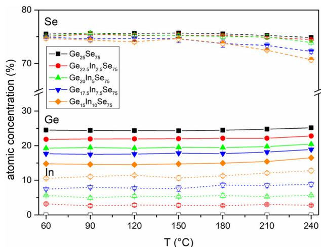
Fig. 2 The elemental composition of prepared  $\text{Ge}_{25-x}\text{In}_x\text{Se}_{75}$  ( $x = 0, 2.5, 5, 7.5, \text{ and } 10$ ) thin films as Ge : In : Se ratio (excluding the light elements) in dependence on hard-baking temperature.
