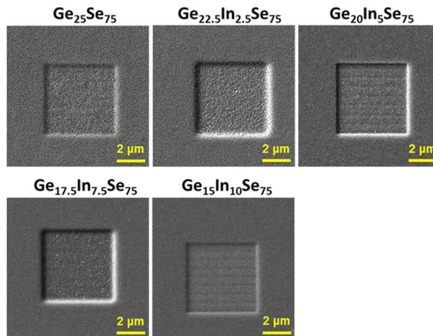
Fig. 11 The SEM scans of EBL patterned  $\text{Ge}_{25-x}\text{In}_x\text{Se}_{75}$  ( $x = 0, 2.5, 5, 7.5$ , and  $10$ ) thin films annealed at  $210^\circ\text{C}$  exposed with a  $750\ \mu\text{C cm}^{-2}$  dose.
