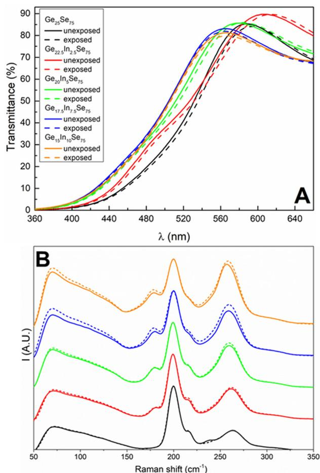
Fig. 7 The transmission (A) and Raman spectra (B) of  $\text{Ge}_{25-x}\text{In}_x\text{Se}_{75}$  ( $x = 0, 2.5, 5, 7.5$  and  $10$ ) thin films annealed at  $210\text{ }^\circ\text{C}$  before (solid line) and after  $532\text{ nm}$  exposure (dashed line).
