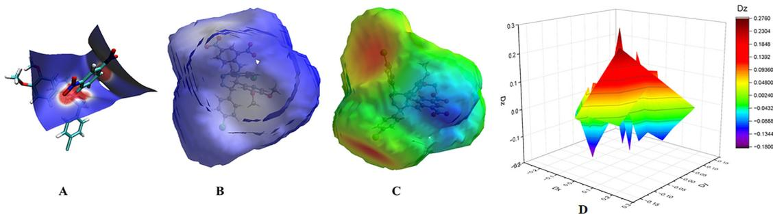
**Fig. 12** (A) Molecular structure of **1c** with the surface, showing that their contact is close (red dots represent strong interactions between molecules); (B) Hirshfeld-mapped shape index showing pi–pi stacking interaction using red and blue triangles; (C) Hirshfeld surface and the property of curviness, where flat regions (green) suggest pi–pi stacking and curved (blue) are regions, edges or corners; and (D) **1c** surface area graph visualization for dipole components.
