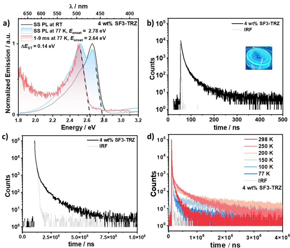
Fig. 4 Photophysical data of the 4 wt% doped film of **Mes-tDABNA** in SF3-TRZ; (a) steady-state PL spectra at room temperature (black) and 77 K (blue) and time-gated emission spectrum (1–9 ms) at 77 K (red) ( $\lambda_{exc} = 340$  nm); (b) time-resolved PL decay under vacuum measured by TCSPC ( $\lambda_{exc} = 375$  nm); (c) time-resolved PL decay under vacuum measured by MCS ( $\lambda_{exc} = 375$  nm); (d) temperature-dependent time-resolved PL decay ( $\lambda_{exc} = 375$  nm).
