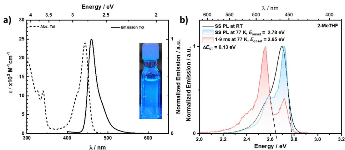
Fig. 3 Absorption and PL spectra of dilute solutions of **Mes-tDABNA**; (a) absorption (dashed) and PL spectra (solid) of **Mes-tDABNA** in dilute ( $\times 10^{-5}$  M) toluene solution ( $\lambda_{\text{exc}} = 340$  nm); (b) steady-state PL spectra of **Mes-tDABNA** in dilute 2-MeTHF solution/glass at room temperature (black) and 77 K (blue), time gated (1–9 ms) PL spectrum of **Mes-tDABNA** in 2-MeTHF glass (red) ( $\lambda_{\text{exc}} = 340$  nm).
