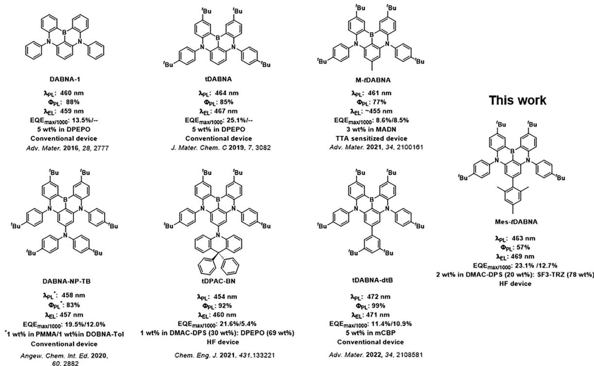
Fig. 1 Chemical structures, photophysical properties and device performance of **Mes-tDABNA** and examples of **tDABNA** derivatives in literature.<sup>10–15</sup>
