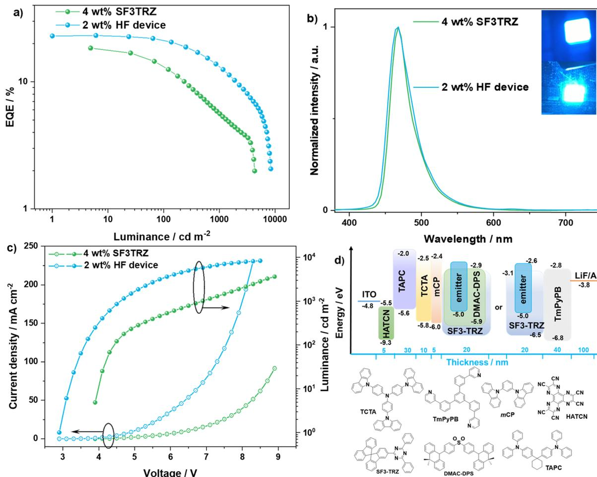
Fig. 5 Device data of **Mes-tDABNA** (green = conventional device) (blue = HF device) (a) EQE vs. luminance plot; (b) electroluminescence spectra; (c)  $J$ - $V$ - $L$  plot (d) device structure and chemical structures of used materials.
