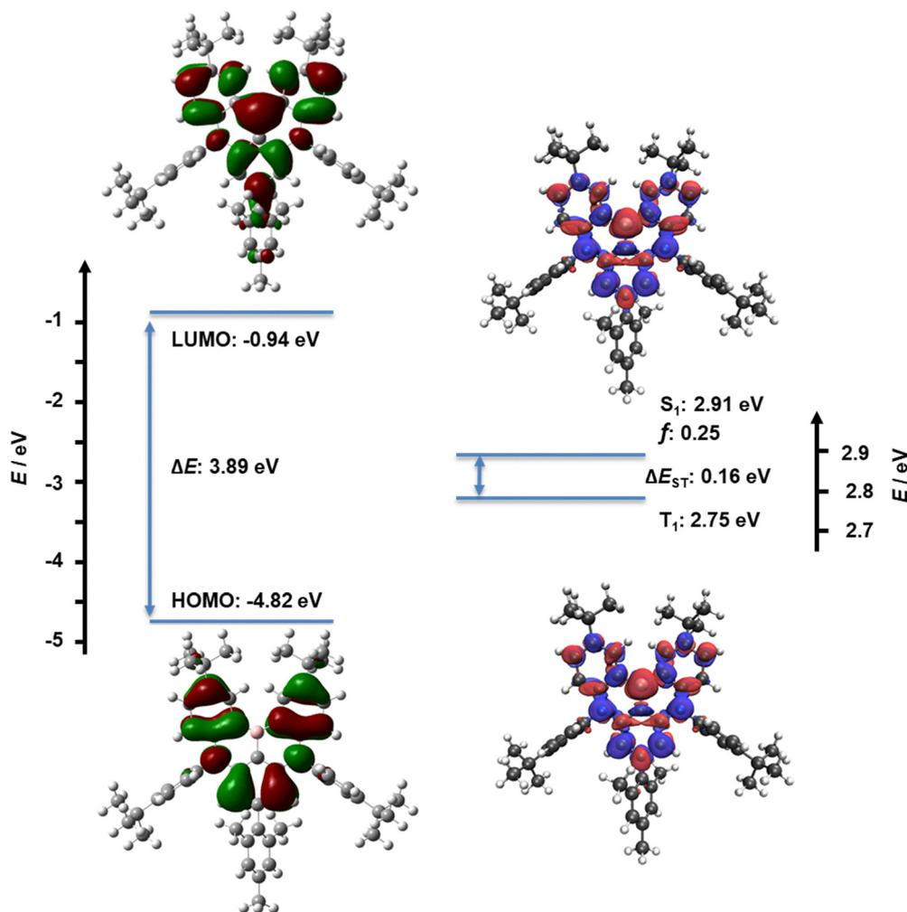
Fig. 2 Calculated HOMO and LUMO energies and the electron density plots calculated of **M-tDABNA** at the PBE0/6-31G(d,p) level in the gas phase and calculated excited-state energies and the corresponding difference density plots for hole and electron for the  $S_1$  and  $T_1$  states at the SCS-ADC(2)/cc-pVDZ level in the gas phase (blue: negative, red: positive, isovalue: 0.02).
