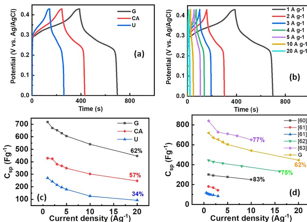
Fig. 7 (a) GCD curves at a current density of  $1 \text{ A g}^{-1}$ , (b) GCD curves of the G sample, (c) specific capacitance vs. current density, and (d) comparison of the capability rate with other reported works.<sup>45–48</sup>
