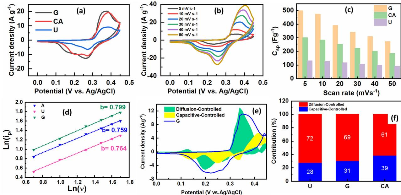
Fig. 6 (a) CV curves at a scan rate of  $5 \text{ mV s}^{-1}$ , (b) CV curves of the G electrode, (c) specific capacitance versus scan rate, (d)  $\ln(i_p)$  vs.  $\ln(\nu)$  plot, (e) capacitive- and diffusion-controlled CV curves, and (f) the contribution ratio of various electrodes.
