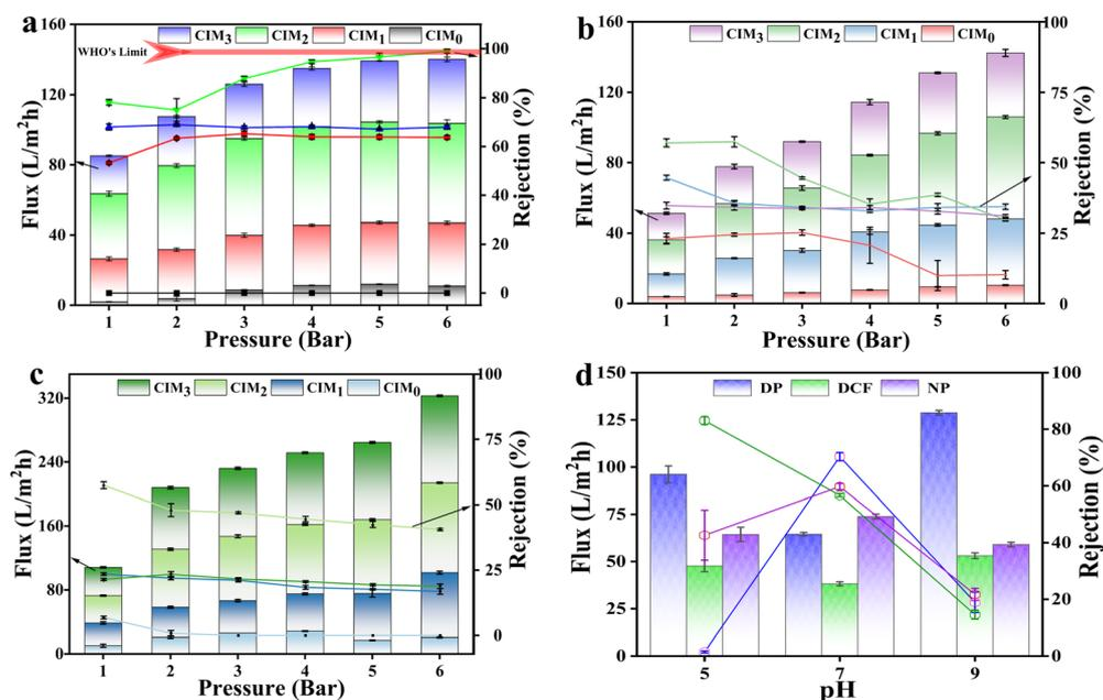
Fig. 6 Flux-rejection graphs of (a) DP, (b) DCF, and (c) NP for MOF-membranes. (d) Effect of pH on the rejection trend (for the optimized CIM<sub>2</sub> membrane).
