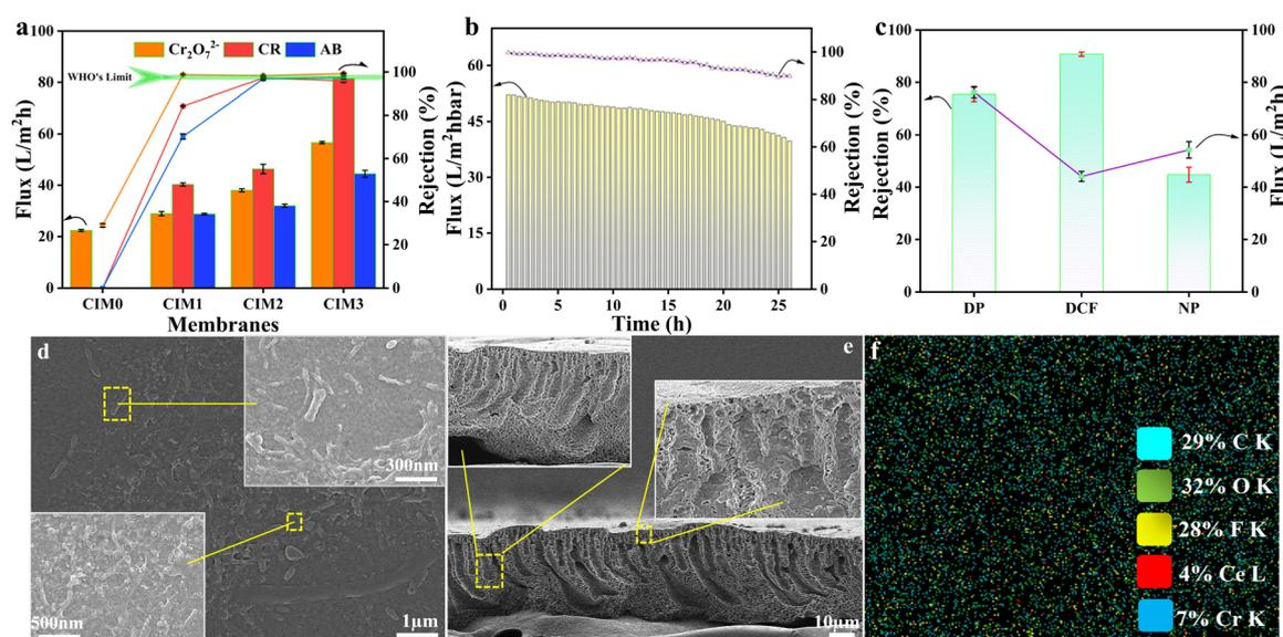
Fig. 7 (a) Flux-rejection graphs of Cr<sub>2</sub>O<sub>7</sub><sup>2-</sup>, AB & CR. (b) Long-term stability. (c) Filtration of SE (for optimized CIM<sub>2</sub> membrane). (d) and (e). FESEM surface and cross-sectional images of CIM<sub>2</sub> after long-term run (insets at a higher magnification).
