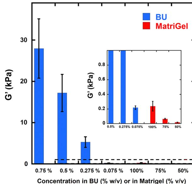
**Fig. 2** Elastic moduli ( $G'$ ) values recorded at a sweep frequency of 1 Hz.  $G'$  of GNBA (BU) based supramolecular gels (blue) versus matrigel (red) are reported at different concentrations (BU % w/v, Matrigel % v/v).
