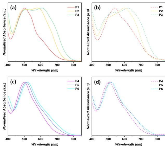
Fig. 2 Normalized UV-vis absorption spectra of copolymers in dilute ( $\sim 10^{-5}$  M) chloroform solution and thin-film state. (a), (b) NDI-based copolymers (**P1–P3**) in solution and film, respectively. (c), (d) PDI-based copolymers (**P4–P6**) in solution and film, respectively.
