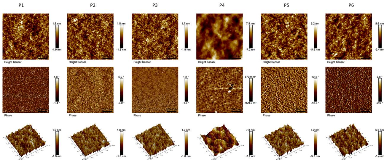
Fig. 6 Atomic Force Microscopy (AFM) tapping mode images recorded over a scan area of  $1 \times 1 \mu\text{m}^2$  of thin films of **P1–P6** showing topography (height sensor, top row), phase (middle row), and corresponding 3D height profiles (bottom row).
