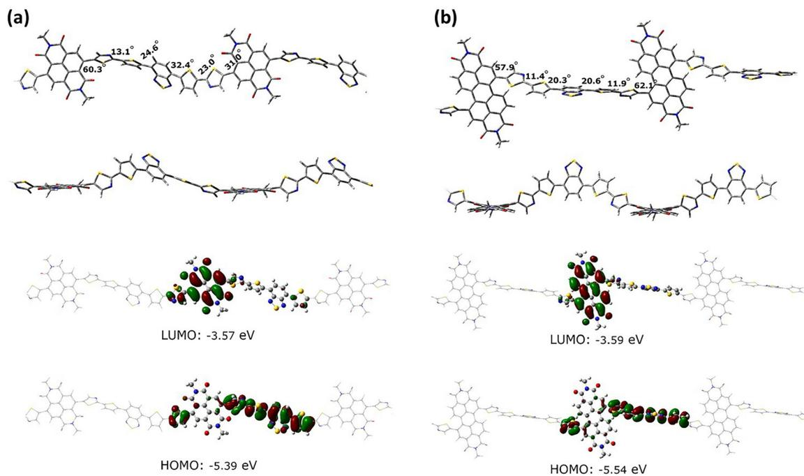
Fig. 4 Representative examples of optimized ground-state structures of copolymers **P1** and **P4** as calculated at the B3LYP/6-31G(d,p) level of theory, with the periodic boundary conditions (PBC). For clarity the HOMO and LUMO orbitals are graphically presented over the single repeat unit.
