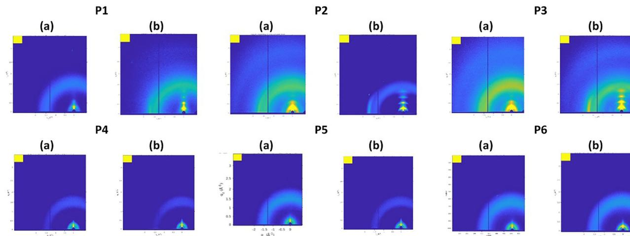
Fig. 5 GIWAXS patterns of **P1–P6** films deposited on silicon wafer substrates (a) as cast (b) annealed films.
