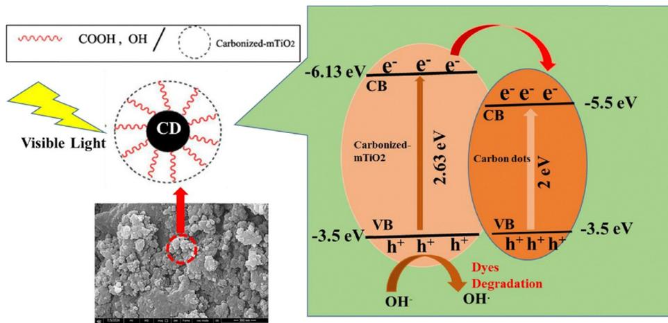
Fig. 5 A schematic illustrating the processes of charge transfer and free radical formation in CD@C-mTiO<sub>2</sub> composites that drive their photocatalytic activity. Reproduced with permission from ref. 61. Copyright 2022, Elsevier.
