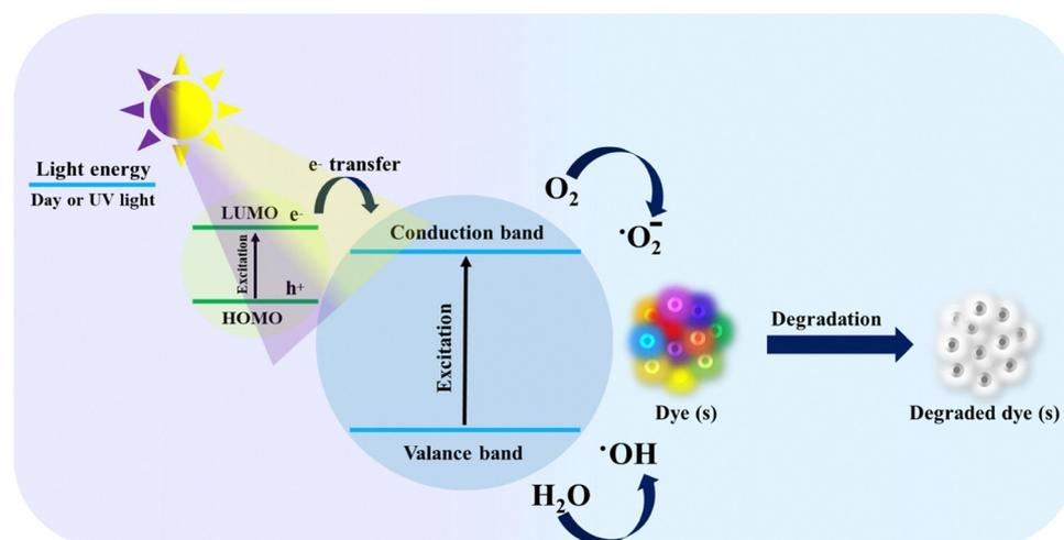
Fig. 4 Schematic representation of the photocatalytic dye removal process by CD/MO hybrid materials.
