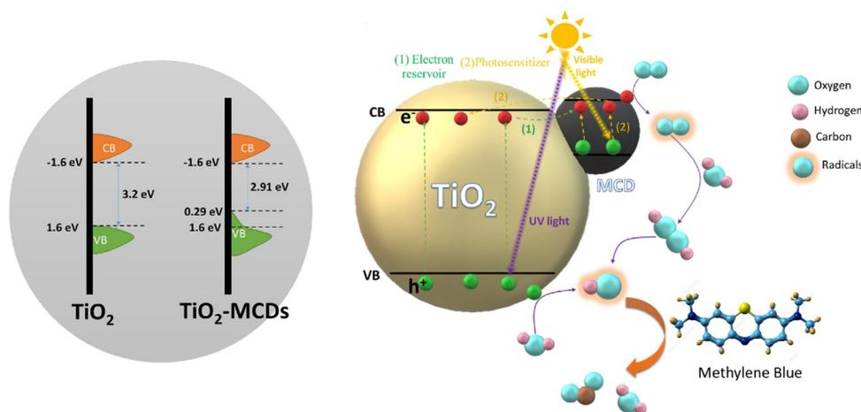
Fig. 6 A schematic depiction of the photocatalytic mechanism demonstrated by TiO<sub>2</sub>-MCDs. Reproduced with permission from ref. 140. Copyright 2022, Elsevier.
