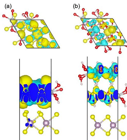
Fig. 10 Top and side views of the spin density distributions of the (a) monolayer  $\beta$ -NiOOH on MoS<sub>2</sub> and (b) bilayer  $\beta$ -NiOOH on MoS<sub>2</sub>. The purple, yellow, grey, red and white balls represent Mo, S, Ni, O, and H, respectively. The black line represents the unit cell boundary.
