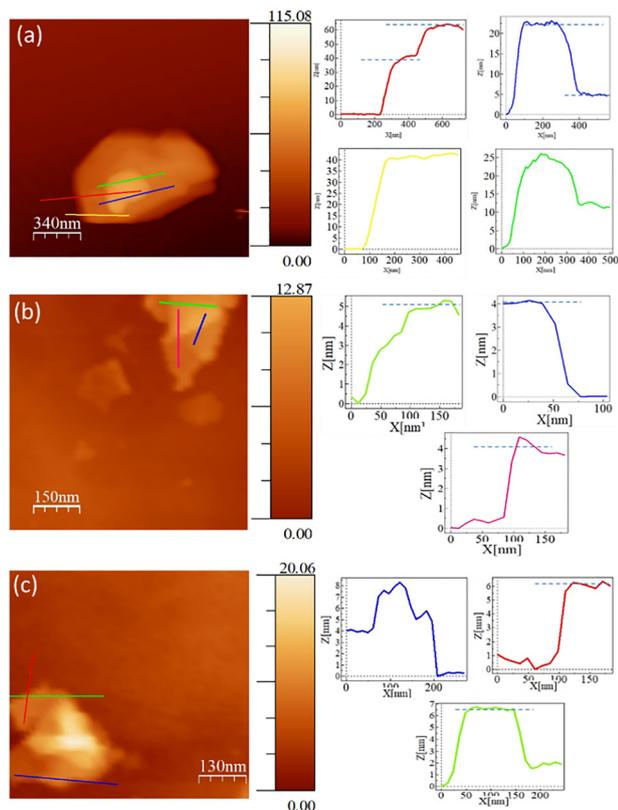
Fig. 4 (a) AFM image of MN-1 with the height profiles of the  $\beta$ -NiOOH layers on the right. The step-like behavior of the typical multilayered heterostructure (MN-1). (b) For MN-2, the thin layer of  $\beta$ -NiOOH can be seen with the average height profile plot shown on the right. (c) For the overall plot of MN-2, with the height profile in the inset showing the average thickness of the grown structures. See SI for the surface topography detailed analysis Section 4.
