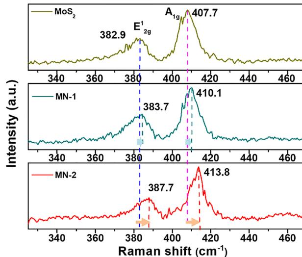
Fig. 3 Raman spectra of the two composites along with the pristine MoS<sub>2</sub> phase for comparison of peak shifting and strain analysis. The position of E<sub>2g</sub><sup>1</sup> and A<sub>1g</sub> are shifted with respect to the pure MoS<sub>2</sub> phase, and the dashed line shows the position with the shift in the composite samples.
