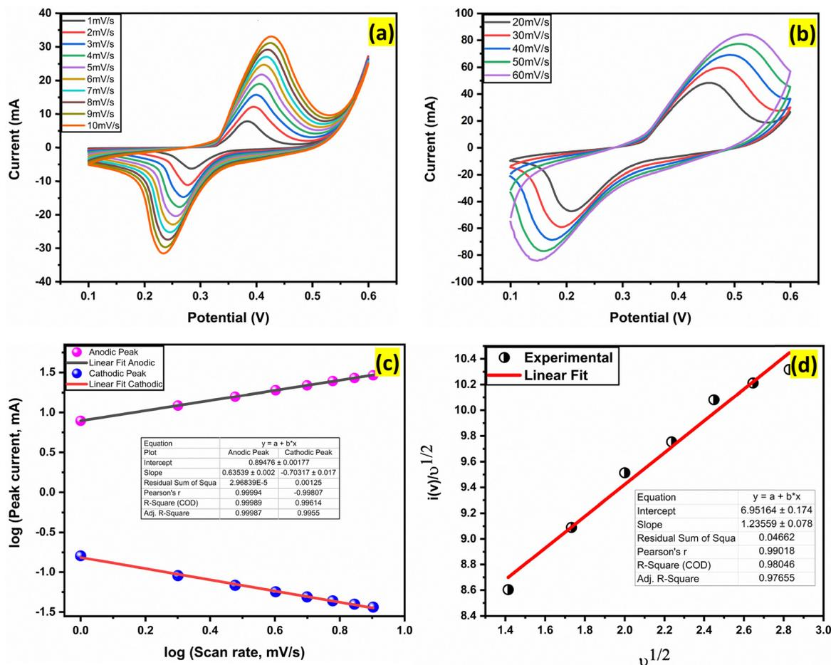
Fig. 8 (a) and (b) Cyclic voltammetry (CV) curves of Alv-ZnO NSs at various scan rates. The specific capacitance was calculated using eqn (9), where  $m$  is the mass of active material (1.5 mg), (c) anodic and cathodic peaks and (d) plot of  $i(V)/v^{1/2}$  vs.  $v^{1/2}$  (where  $v$  is scan rate).
