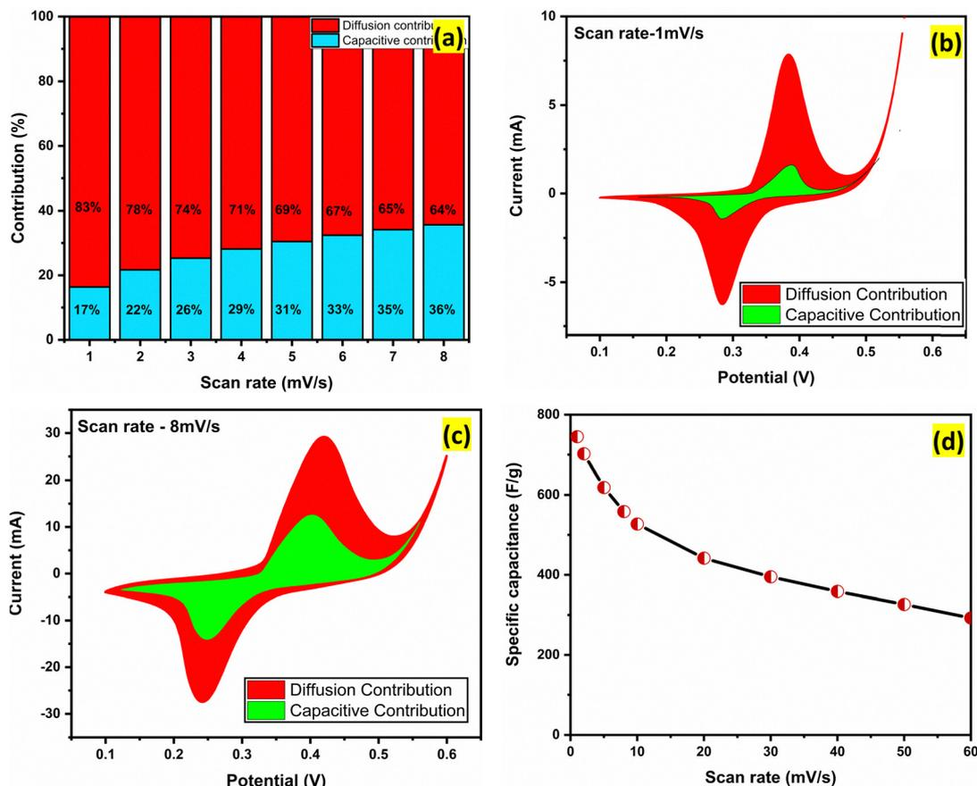
Fig. 9 (a) Bar diagram showing the capacitive and diffusion contributions to the overall current at varying scan rates. (b) and (c) CV profiles at  $1 \text{ mV s}^{-1}$  and  $8 \text{ mV s}^{-1}$  scan rates, illustrating the capacitive contribution at two different scan rates. (d) Specific capacitance vs. scan rate trend for the AlV-ZnO NSs, showing the variation in capacitance with changing scan rate.
