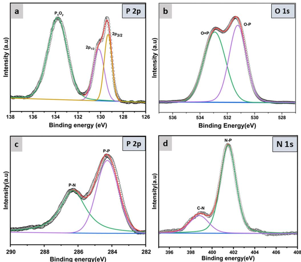
Fig. 6 (a) High-resolution XPS spectrum of BP-200 with P 2p peaks corresponding to  $P_2O_5$  (oxidized phosphorus) and  $P^\circ$  (elemental phosphorus). (b) O 1s spectrum showing contributions from O=P and O-P bonds, indicative of surface oxidation. (c) C 1s spectrum with peaks corresponding to P-N and P-P bonding. (d) N 1s spectrum highlighting N-P and C-N bonding.
