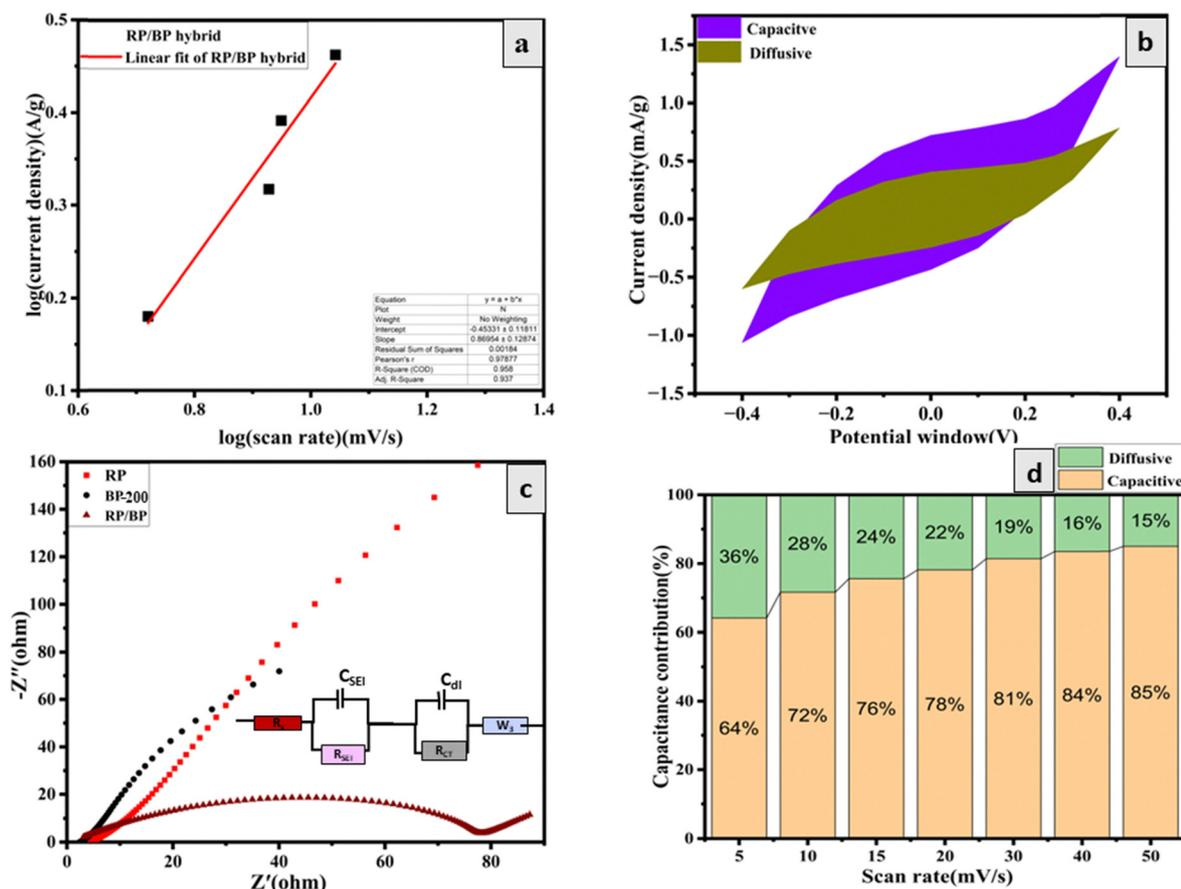
Fig. 9 (a) Linear fit for “b” value. (b) Capacitance contribution analysis in the RP/BP hybrid via CV at  $0.5 \text{ mV s}^{-1}$ . (c) Nyquist plots of RP, BP, and the RP/BP hybrid with Randles circuit. (d) Capacitance contribution in the RP/BP hybrid using the Dunn method.
