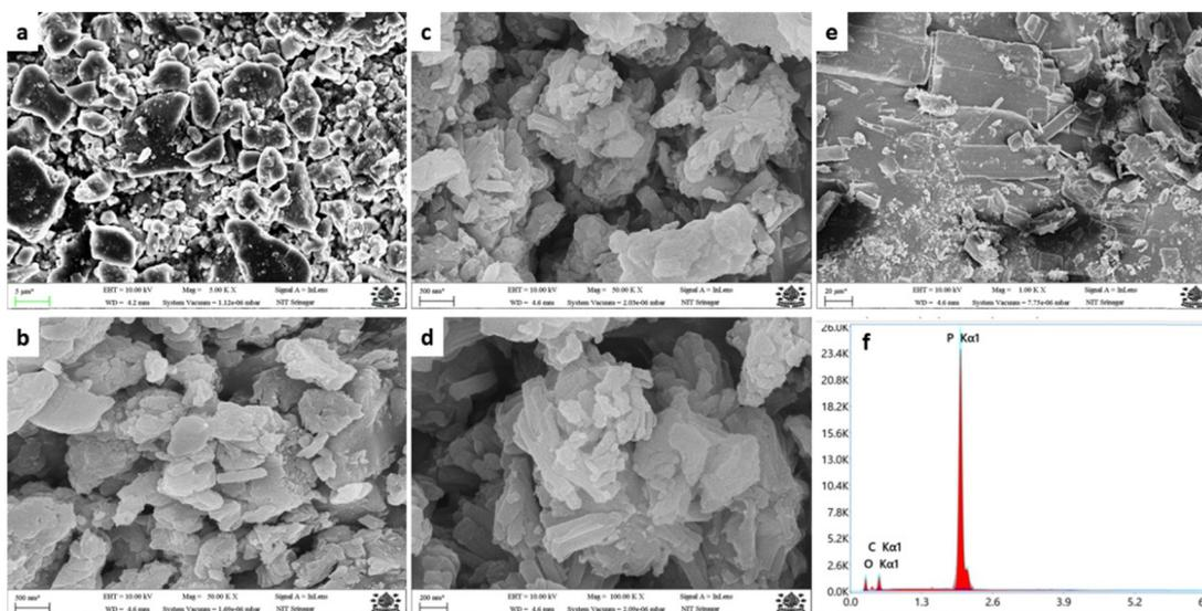
Fig. 5 (a) RP SEM picture exhibiting irregular microstructures without layers. (b) SEM picture of BP-160 BP showing multilayer structures. (c) SEM picture of BP-180 showing enhanced layer consistency and stacking. (d) SEM picture of BP-200 showing layer hierarchy. (e) Magnified SEM picture of BP-200 with well-defined exfoliated layers. (f) EDX of BP-200.
