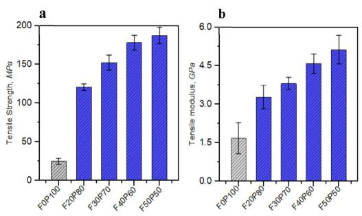
Fig. 4 Tensile properties of UD jute-PLA biocomposites with respect to fibre weight fraction: (a) tensile strength of composites and (b) tensile modulus of composites.
