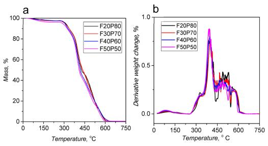
Thermal analysis of jute/PLA biodegradable composites: (a) TGA analysis and (b) DTG analysis
