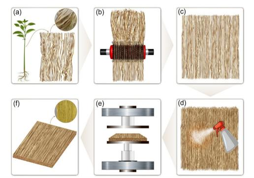
Fig. 1 Schematic of preform (UD) preparation: (a) raw long jute from jute plants, (b) fibre hackling process, (c) aligning long jute, (d) applying 1% starch, (e) compression moulding, and (f) jute fibre preform.
