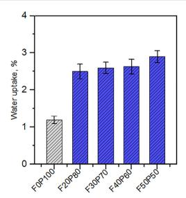
Fig. 6 Water uptake percentage of UD jute-PLA biocomposites with respect to fibre content.
