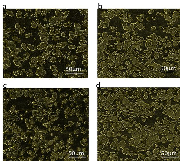
Fig. 7 Optical micrographs of the different composites 250 $\times$  magnification: (a) composite cross section at 20% fiber content, (b) composite cross section at 30% fiber content, (c) composite cross section at 40% fiber content, and (d) composite cross section at 50% fiber content.
