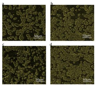
Optical micrographs of the different composites 250× magnification: (a) composite cross section at 20% fiber content, (b) composite cross section at 30% fiber content, (c) composite cross section at 40% fiber content, and (d) composite cross section at 50% fiber content
