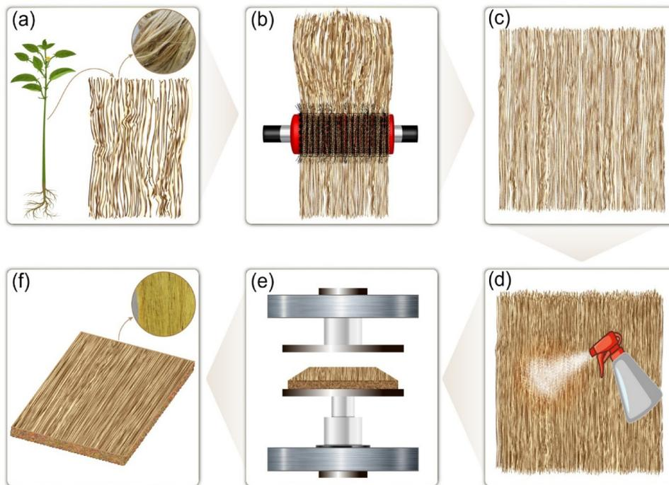
**Fig. 1** Schematic of preform (UD) preparation: (a) raw long jute from jute plants, (b) fibre hackling process, (c) aligning long jute, (d) applying 1% starch, (e) compression moulding, and (f) jute fibre preform.
