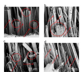
Fig. 8 SEM micrograph of UD jute-PLA biocomposites tensile fractured specimens: (a) fracture specimen of F20P80 composites, (b) fracture specimen of F30P70 composites. (c) fracture specimen of F40P60 composites, and (d) fracture specimen of F50P50 composites.
