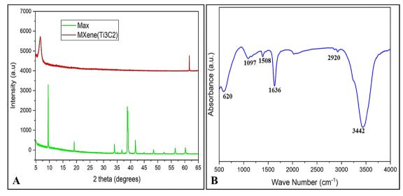
Fig. 3 Characteristics study: (A) XRD of the Max phase ( $Ti_3AlC_2$ ) and delaminated MXene sheets ( $Ti_3C_2X$ ) and (B) FTIR of delaminated MXene sheets ( $Ti_3C_2X$ ).
