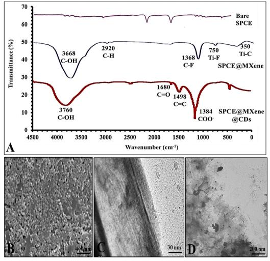
Fig. 4 SPCE characteristics study: (A) FTIR spectra of bare SPCE, SPCE@MXene, and SPCE@MXene@CDs and (B) HRTEM images of bare SPCE, SPCE@MXene, and SPCE@MXene@CDs.
