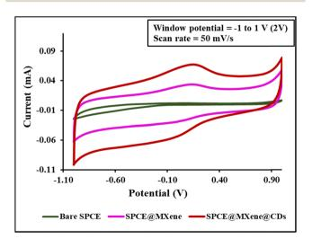
Fig. 6 CV characterization of bare SPCE, SPCE@MXene, and SPCE@M-Xene@CDs was performed in a 0.1 M PBS solution (pH 7) at a scan rate of 50 mV s<sup>-1</sup>, using an Ag/AgCl reference electrode
