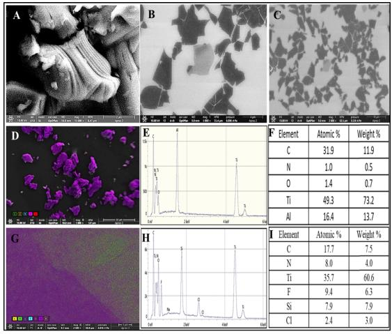
Fig. 2 Microscopic characterization of MXene: HR-SEM for (A) the Max phase  $(Ti_3AlC_2)$  and (B) and (C) delaminated MXene sheets  $(Ti_3C_2X)$ ; EDS analysis: (D) EDS image, (E) EDS mapping, and (F) elemental composition of the Max phase  $(Ti_3AlC_2X)$ ; (G) EDS image, (H) EDS mapping, and (I) elemental composition of delaminated MXene sheets  $(Ti_3C_2X)$ .
