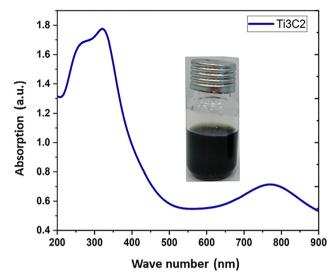
Fig. 1 UV-Visible characteristics of delaminated MXene sheets (Ti<sub>3</sub>C<sub>2</sub>X).
