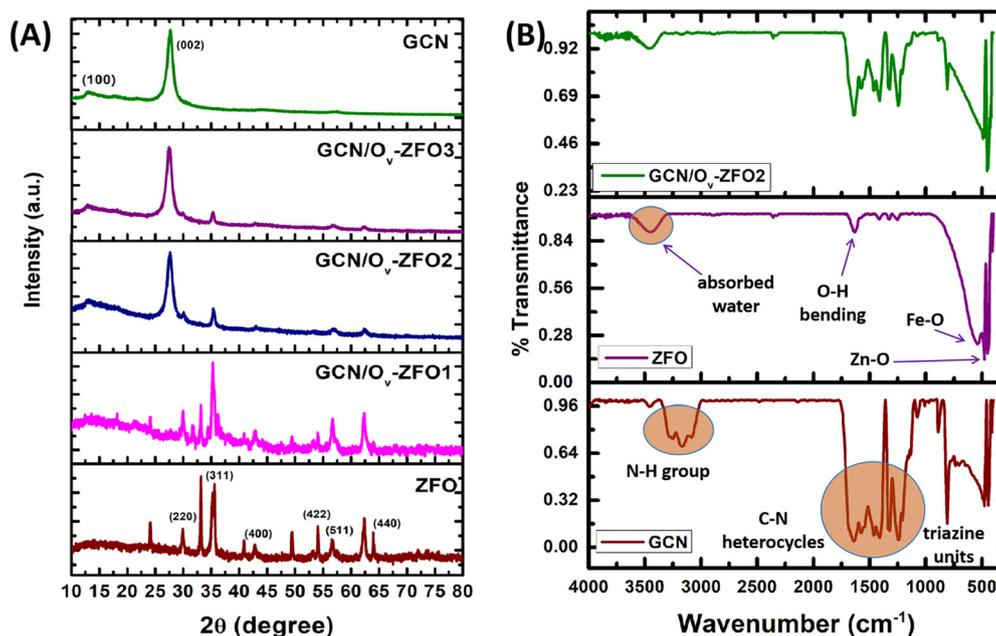
Fig. 1 (A) X-ray diffraction peaks of the as-prepared samples and (B) FTIR spectra of GCN, ZFO and GCN/O<sub>v</sub>-ZFO<sub>2</sub>.
