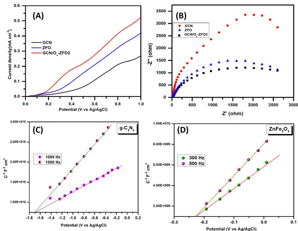
Fig. 7 (A) LSV and (B) EIS plots of GCN, ZFO and GCN/O<sub>v</sub>-ZFO2, and MS plots of (C) GCN and (D) ZFO.
