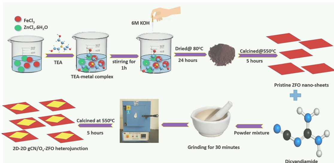
Scheme 1 Schematic representation of the detailed synthesis protocol for the GCN/O<sub>v</sub>-ZFO heterojunction.
