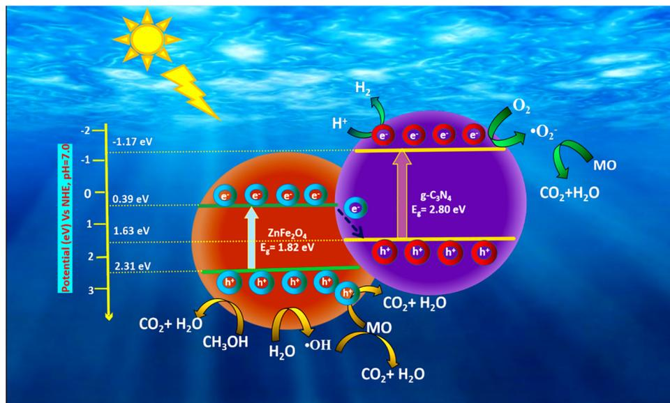
**Scheme 2** Diagrammatic representation of photocatalytic H<sub>2</sub> production and MO degradation using the 2D–2D GCN/O<sub>v</sub>–ZFO<sub>2</sub> direct Z-scheme heterojunction nanocomposite.
