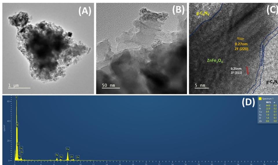
Fig. 4 TEM micro-graph at different resolutions (A) and (B), respective HRTEM image (C) and EDX spectrum (D) of GCN/O<sub>v</sub>-ZFO<sub>2</sub>.
