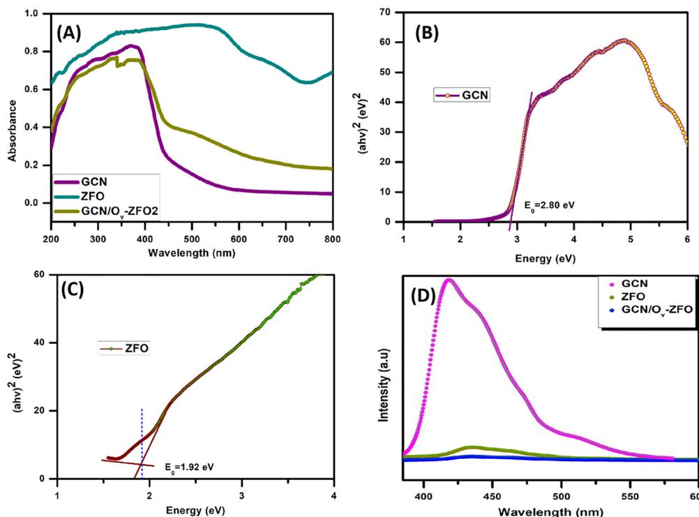
Fig. 6 (A) UV-Visible DRS spectra of GCN, ZFO and GCN/O<sub>v</sub>-ZFO2, estimated band gaps of (B) GCN and (C) ZFO, and (D) PL emission spectrum of ZFO and GCN/O<sub>v</sub>-ZFO2.
