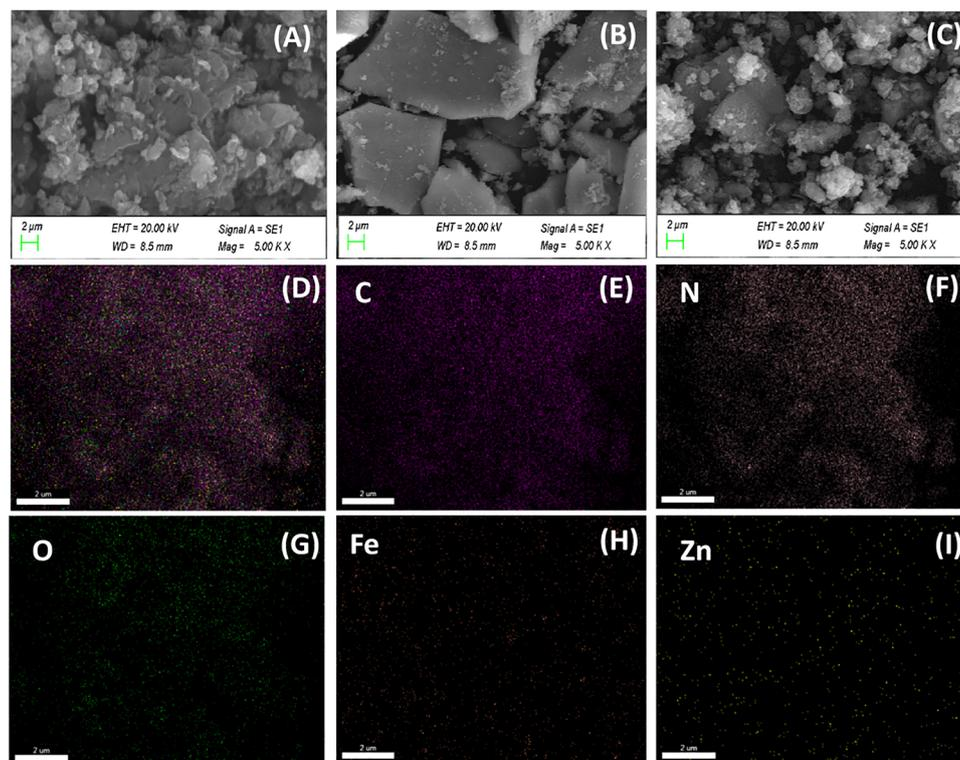
Fig. 3 SEM images of (A) GCN, (B) ZFO, (C) GCN/ $\text{O}_v$ -ZFO<sub>2</sub> and elemental the colour mapping image of (D) GCN/ $\text{O}_v$ -ZFO<sub>2</sub> showing the homogeneous distribution of (E) carbon, (F) nitrogen, (G) oxygen, (H) iron and (I) zinc.
