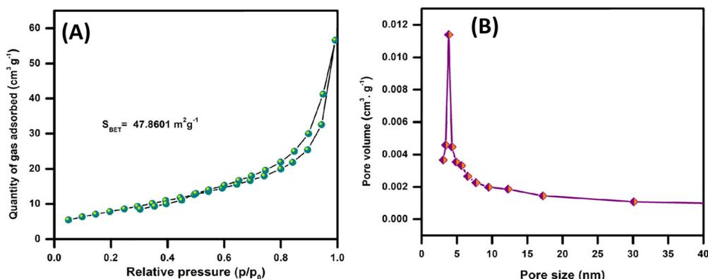
Fig. 5 (A) BET specific surface area and (B) BJH pore size distribution curve of GCN/O<sub>v</sub>-ZFO<sub>2</sub>.
