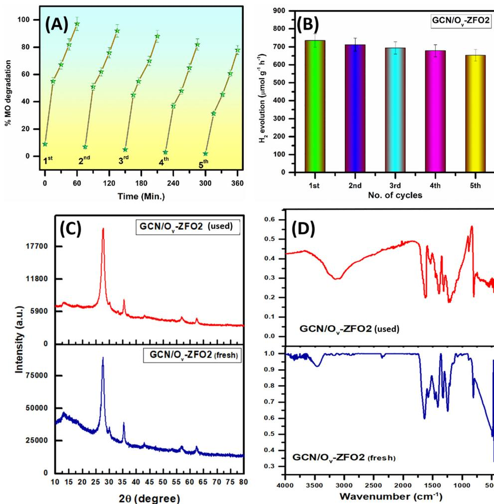
Fig. 9 Photocatalytic (A) MO degradation curves and (B) rate of H<sub>2</sub> evolution in the reusability test of the GCN/O<sub>v</sub>-ZFO2 catalyst for five consecutive cycles, and comparison of (C) XRD and (D) FTIR spectrum of fresh and used GCN/O<sub>v</sub>-ZFO2 catalysts.
