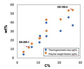
**Fig. 6** Polymer weight fractions (wt%) of POSS–DMS grafted silicas, determined by <sup>29</sup>Si NMR and TGA (weight loss at 900 °C) as a function of carbon content (C%) obtained from elemental analysis.
