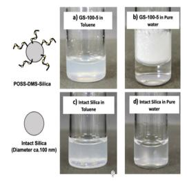
Fig. 3 Photographs of the dispersed states of POSS-DMS-grafted silica (a) and (b) and intact silica (GS-100-5); (c) and (d) in toluene (a) and (c) and pure water (b) and (d).
