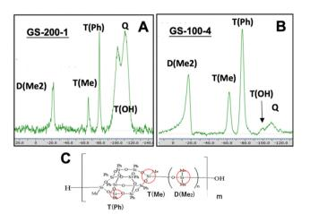
Fig. 5  $\,^{29}$ Si-NMR spectra of GS-200-1 (A) and GS-100-4 (B), and chemical structure of POSS-DMS polymers for NMR assignments (C).
