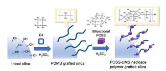
Fig. 1 Schematic representation of the two-step ring-opening equilibrium polymerization for POSS-DMS necklace-shaped, polymer-grafted
