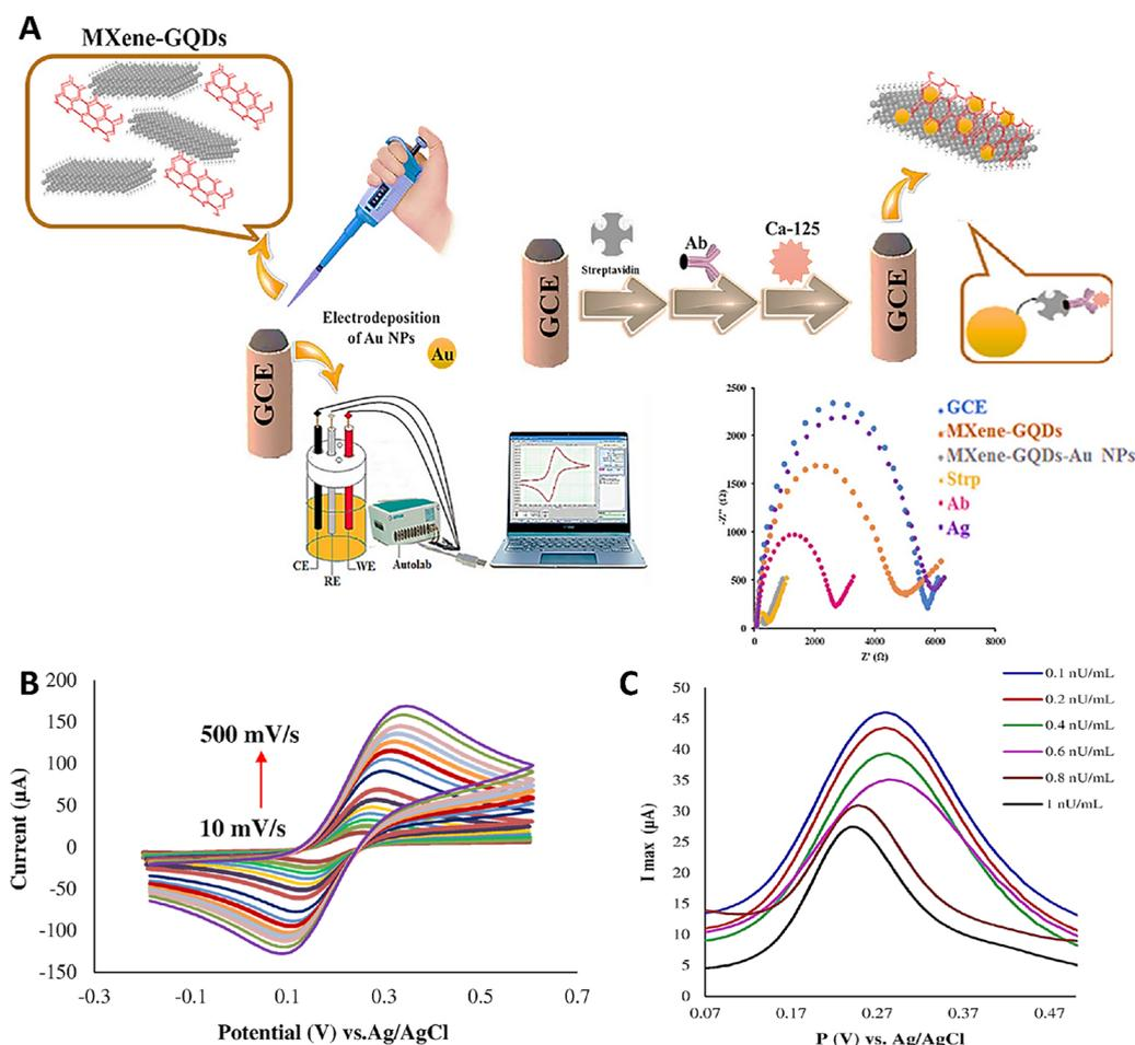
**Fig. 1** (A) Schematic image of fabrication process of MXene-GQD/AuNPs immunosensor. (B) Results of sensing kinetic of fabricated sensor in the presence of different scan rates ( $10$ – $500 \text{ mV s}^{-1}$ ). (C) Detection of different concentrations of CA125 in real sample. Reprinted with permission from ref. 137. Copyright 2024, The Author(s).
