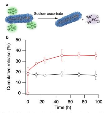
Fig. 4 (a) Schematic illustration of platinum catalyst release from cylindrical micelles in the presence of sodium ascorbate. (b) Cumulative release of the platinum catalyst from cylindrical micelles in the presence (red circles) and absence (gray circles) of sodium ascorbate at 25 °C.
