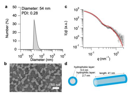
Fig. 2 (a) Size distribution of self-assembled PAA-g-PPO (1.0 mg mL<sup>-1</sup>) in PBS. (b) TEM image of self-assembled PAA-g-PPO with negative staining phosphotungstic acid. (c) SAXS profile of self-assembled PAA-g-PPO (open circles) in PBS at 25 °C and the theoretical curve obtained using the coreshell cylinder model (red line). (d) The structural parameters of the cylindrical micelles.
