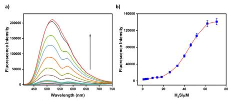
Fig. 8 (a) Emission behaviour of BHS-Cu<sup>2+</sup> ( $c = 2 \times 10^{-5}$  M) with the addition of H<sub>2</sub>S solution ( $c = 2 \times 10^{-4}$  M). (b) Emission intensity changes of the BHS-Cu<sup>2+</sup> complex as a function of the H<sub>2</sub>S concentration.
