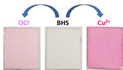
Fig. 9 Color changes of the BHS-treated TLC plates ( c = 2 \times 10^{-5} M) with an exposure to \text{Cu}^{2+} and \text{OCl}^- ( c = 2 \times 10^{-4} M).
