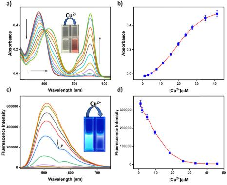
Fig. 1 (a) and (c) Colorimetric and fluorometric response of **BHS** ( $c = 2 \times 10^{-5}$  M) with the addition of Cu<sup>2+</sup> ( $c = 2 \times 10^{-4}$  M, 10 equiv.). (b) and (d) Changes in concentrations vs. intensity of **BHS** with  $Cu^{2+}$  in absorption and emission titration spectra, respectively ( $\lambda_{em} = 576$  nm).
