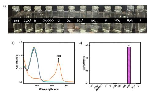
Fig. 5 (a) The changes of naked eye color of the probe **BHS** with several anions. (b) Absorption behaviour of **BHS** upon addition of several anions (10 equiv.) in CH<sub>3</sub>CN-aqueous HEPES buffer solution (9/1, v/v, pH = 7.4). (c) Absorption intensity changes of the probe **BHS** upon the addition of interfering anions ( $c = 2 \times 10^{-4}$  M, 10 equiv.).
