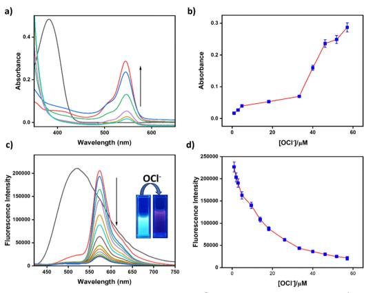
Fig. 2 (a) and (c) Absorption and emission titration signals of **BHS** ( $c = 2 \times 10^{-5}$  M) with the addition of OCl<sup>-</sup> ( $c = 2 \times 10^{-4}$  M, 10 equiv.). (b) and (d) Concentrations vs. intensity variations of **BHS** with OCl<sup>-</sup> in colorimetric and fluorometric titration spectra, respectively ( $\lambda_{em} = 576$  nm).
