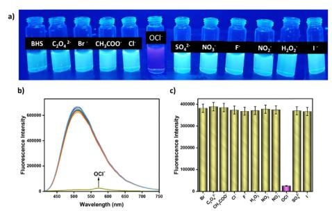
Fig. 6 (a) Fluorescent properties of ligand BHS with different anions under UV light. (b) The fluorescence spectra of BHS with the addition of several anions (10 equiv.) in CH<sub>3</sub>CN-aqueous HEPES buffer solution (9/1, v/v, pH = 7.4). (c) Changes of fluorescence intensity of the sensor **BHS** with the addition of various interfering anions ( $c = 2 \times 10^{-4}$  M, 10 equiv.).
