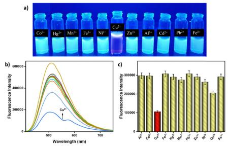
Fig. 4 (a) Fluorescent properties of probe **BHS** with various cations under UV light. (b) Fluorescence signal of **BHS** on the addition of various cations (10 equiv.) in CH<sub>3</sub>CN-aqueous HEPES buffer solution (9/1, v/v, pH = 7.4). (c) Changes in fluorescence intensity of the sensor **BHS** with the addition of other interfering cations ( $c = 2 \times 10^{-4}$  M, 10 equiv.).
