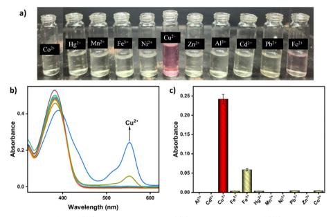
Fig. 3 (a) Naked eye colour changes of probe BHS with several metal ions. (b) Colorimetric behaviour of BHS on exposure to diverse metal ions (10 equiv.) in CH<sub>3</sub>CN-aqueous HEPES buffer solution (9/1, v/v, pH = 7.4). (c) Absorption intensity changes of the sensor **BHS** upon introduction of the interfering metal ions ( $c = 2 \times 10^{-4}$  M, 10 equiv.).
