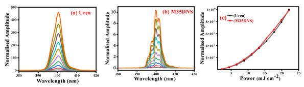
Second harmonic generation comparison of (a) urea, (b) M35DNS, and (c) M35DNS and urea.
