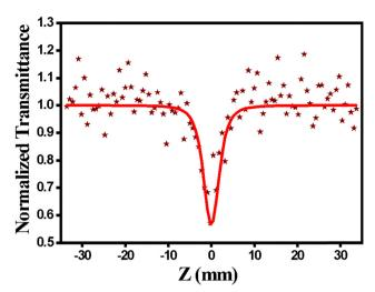
Fig. 14 Open aperture pattern of M35DNS.
