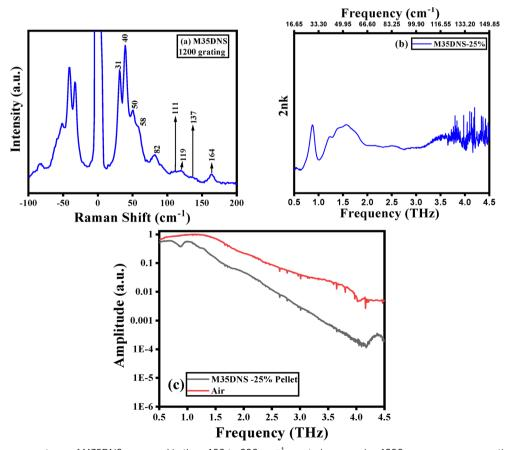
Fig. 13 (a) THz-Raman spectrum of M35DNS measured in the -100 to  $200 \text{ cm}^{-1}$  spectral range using 1200 grooves per mm grating with an exposure time of 5 seconds and 20 accumulations. (b) Variation of 2nk with frequency ranging from 0.5 to 4.5 THz. (c) Amplitude variation of air and M35DNS in the 0.5–4.5 THz spectral range obtained using time domain-THz spectroscopy.
