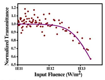
Fig. 15 Optical limiting curves for M35DNS
