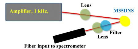
Fig. 11 Second harmonic generation setup
