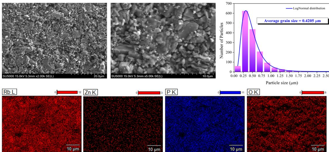
**Fig. 3** Microstructural and compositional analysis of RbZnPO<sub>4</sub> synthesized by solid-state reaction and recorded at room temperature. (top left & middle) SEM images at different magnifications showing a polycrystalline microstructure. (top right) Grain size distribution fitted with a log-normal function, revealing an average grain size of 0.4205 μm. (bottom row) EDS elemental mapping of Rb, Zn, P, and O.
