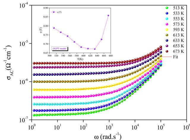
Fig. 10 Frequency dependence of AC conductivity ( $\sigma_{\text{AC}}$ ) versus angular frequency ( $\omega$ ). Inset: Temperature dependence of the frequency exponent  $s(T)$ , showing non-monotonic behavior consistent with OLPT model.
