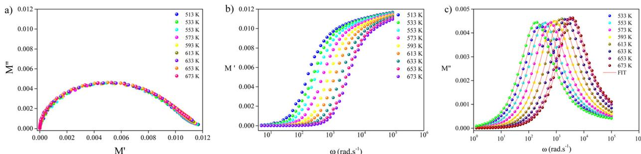
Fig. 5 Electrical modulus analysis of RbZnPO<sub>4</sub> in the 513–673 K temperature range. (a) Complex modulus plot ( $M''$  vs.  $M'$ ); (b) frequency dependence of modulus' ( $M'$ ) real part (c) Frequency dependence of modulus' ( $M''$ ) imaginary part with fitted curves.
