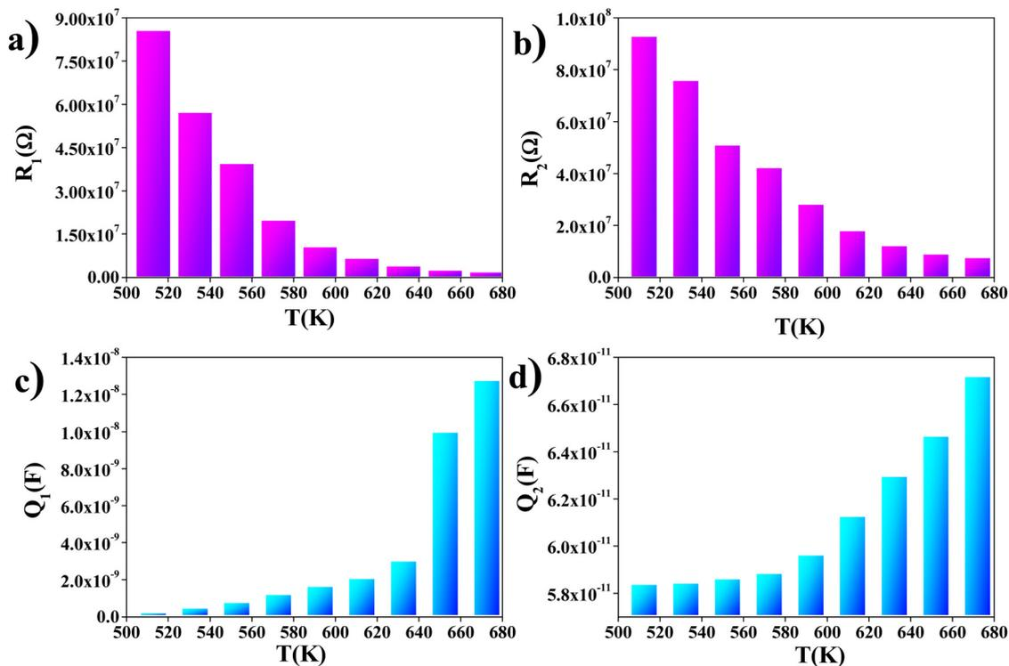
Fig. 7 Temperature dependence of the resistance and constant phase element (CPE) parameters extracted from Nyquist plot fittings: (a) grain resistance  $R_1$ , (b) grain boundary resistance  $R_2$ , (c) grain CPE capacitance  $Q_1$ , and (d) grain boundary CPE capacitance  $Q_2$ .
