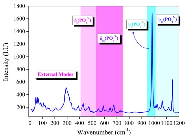
**Fig. 4** Room-temperature Raman spectra of RbZnPO<sub>4</sub> recorded in the 10–1200 cm<sup>-1</sup> Wavenumber range, showing vibrational modes of the [PO<sub>4</sub>]<sup>3-</sup> tetrahedra.
