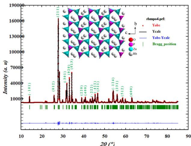
Fig. 1 Room-temperature Rietveld refinement of the X-ray powder diffraction pattern of  $\text{RbZnPO}_4$  compound: experimental (red dotted), Calculated (black line), difference (blue), and Bragg Positions (green bars). Inset: Crystal structure projection along the  $a$ -axis showing the  $bc$ -plane.
