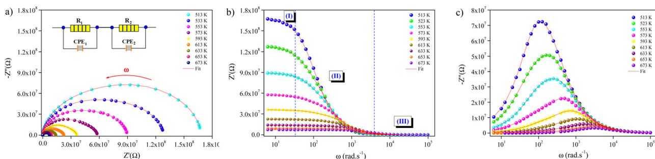
Fig. 6 (a) Nyquist plot of RbZnPO<sub>4</sub> in the 513–673 K temperature range (inset: equivalent circuit model used for data fitting ( $R_1//CPE_1 + R_2//CPE_2$ )), (b) Frequency dependence of real ( $Z'$ ) and (c) imaginary ( $-Z''$ ) parts of complex impedance.
