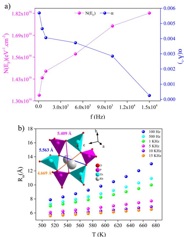
Fig. 12 Variation of (a)  $\alpha$  ( $\text{\AA}^{-1}$ ) and  $N(E_F)$  ( $\text{eV}^{-1} \text{cm}^{-3}$ ) according to the frequency (OLPT model) and (b) temperature-dependence of the tunneling distance  $R_\omega$  ( $\text{\AA}$ ) at different frequencies, supporting the large polaron conduction mechanism.
