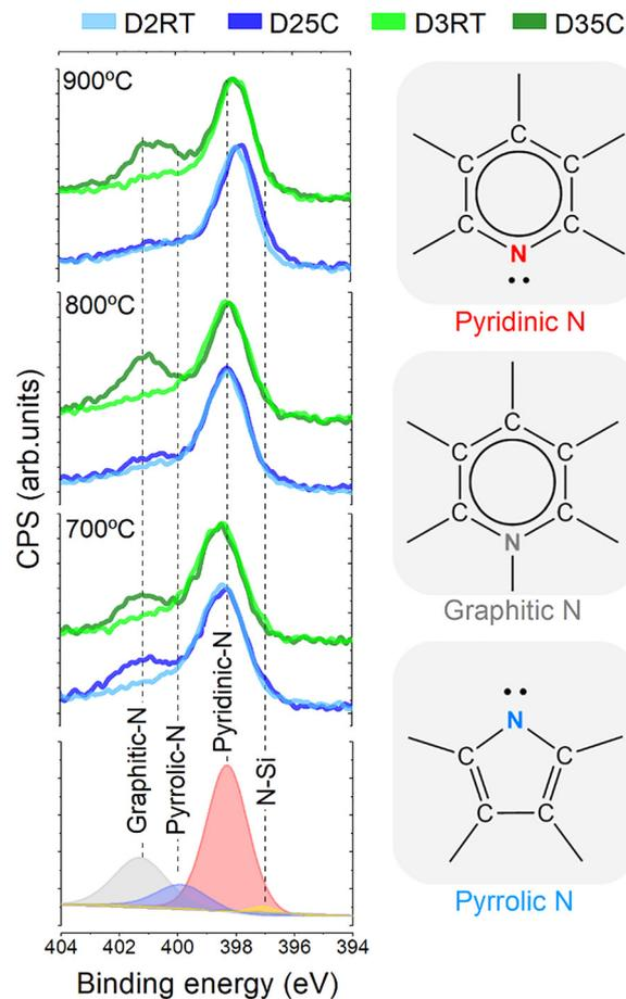
**Fig. 8** High-resolution N 1s XPS spectra of the pyrolyzed materials and their corresponding pseudo-Gaussian deconvolution. This plot highlights the varied nitrogen configurations introduced into the pyrolyzed materials, namely pyridinic-N, graphitic-N and pyrrolic-N, which coexist with N–Si bonds established in the glassy phase.
