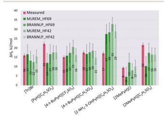
Fig. 5 Predicted *versus* experimental enthalpies of fusion ( $\Delta H_{f_t}$  kJ mol<sup>-1</sup>) for selected organic salt PCMs using four different regression models, highlighting model accuracy in enthalpy estimation.
