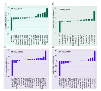
Fig. 4 Scaled regression coefficients of descriptors used in the MLREM models for enthalpy of fusion (a) and (b) and melting temperature (c) and (d).
