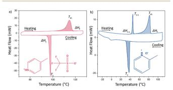
Fig. 2 Differential scanning calorimetry traces of (a) [4-MePyH][CF<sub>3</sub>SO<sub>3</sub>] indicating only one endothermic peak corresponding to melting of the salt, (b) [2-MePyH]Cl showing a solid-solid transition in addition to melting in the heating cycle.
