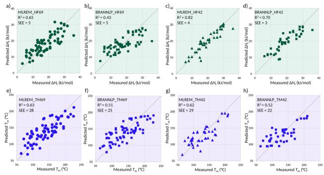
Fig. 3 Comparison of experimental versus predicted melting enthalpies (a)–(d) and melting temperatures (e)–(h) of protic organic salt PCMs according to MLREM and BRANNLP models. The panel ((a) and (b)) and ((e) and (f)) represent models developed using dataset-a (69 datapoints) while panels ((c) and (d)) and ((g) and (h)) represent models developed using dataset-b (42 data points).
