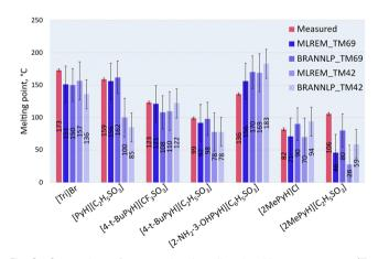
Fig. 6 Comparison of measured and predicted melting temperatures ( $T_{m_l}$ °C) for selected organic salt PCMs across four regression models, demonstrating model performance in melting point prediction.
