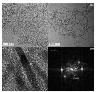
Fig. 1 TEM images of (A) synthesized TiO<sub>2</sub> and of (B) 3% Fe<sub>(doped)</sub><sup>2+</sup>-TiO<sub>2</sub> nanorods. The scale bar is 100 nm (top left and right). (C) High-resolution TEM image of anatase TiO2 nanorods with a scale bar of 5 nm. (D) The highresolution image of the boxed region is shown by fast Fourier transform (FFT).
