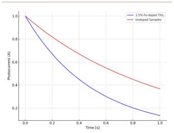
Fig. 13 Photocurrent decay profiles of undoped TiO<sub>2</sub> and 1.5% Fe-doped TiO<sub>2</sub> samples under continuous illumination.
