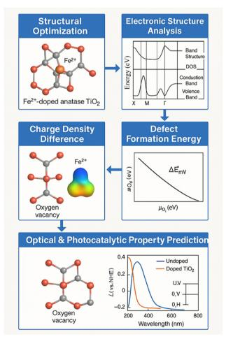
Fig. 10 Proposed mechanism of enhanced photocatalytic activity in Fe<sup>2+</sup>-doped TiO<sub>2</sub> nanorods under visible light irradiation. The illustration highlights Fe<sup>2+</sup> ion incorporation into the TiO<sub>2</sub> lattice via thermal diffusion, the resulting bandgap narrowing, formation of intermediate energy levels, and generation of oxygen vacancies enhancing charge separation and reactive oxygen species production.
