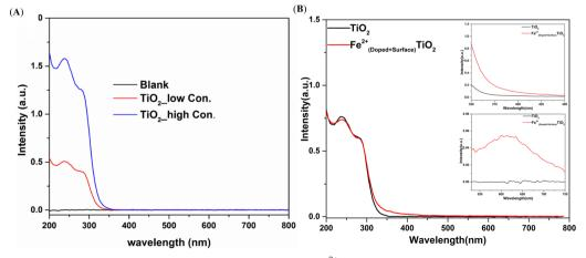
Fig. 3 UV-visible absorption spectra of (A) synthesized  $TiO_2$  and (B) 1.5%  $Fe_{(doped)}^{2+}$  – $TiO_2$  nanorods dispersed in hexane.
