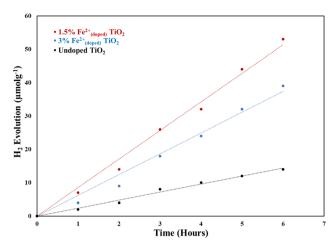
Fig. 9 Time-dependent photocatalytic hydrogen production. Rate of hydrogen generation using 200 W Xe Arc lamp as light source.
