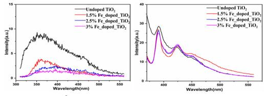
Fig. 6 PL spectra of undoped and  $Fe_{(doped)}^{2+}$ - $TiO_2$  nanocrystals with different dopant concentrations. PL spectra measured with the excitation wavelength at 290 nm (left) and 350 nm (right).
