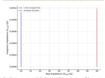
Fig. 12 Nyquist plots of 1.5% Fe-doped  ${\rm TiO_2}$  and undoped  ${\rm TiO_2}$  samples, showing the real ( $Z_{\rm real}$ ) and imaginary ( $Z_{\rm imag}$ ) components of the impedance. The Fe-doped sample exhibits significantly lower impedance, indicating enhanced electrical conductivity and improved charge transport properties due to the incorporation of Fe ions into the  ${\rm TiO_2}$  lattice.
