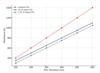
Fig. 8 Resistance versus film thickness plot for thin-film samples of TiO<sub>2</sub> and Fe-doped TiO<sub>2</sub> on ITO-coated glass substrate.
