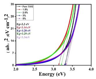
Fig. 7 Tauc plot for prepared Fe-doped TiO<sub>2</sub> nanorods. The plot shows a bandgap range of 3.3-3.1 eV, narrowed by Fe doping, enhancing visible light absorption for photocatalytic and solar applications.
