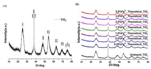
Fig. 2 XRD pattern of (A)  $TiO_2$  nanorods and (B)  $Fe_{(doped)}^{2+}$  – $TiO_2$  samples with different dopant concentrations. The labels indicate the theoretical ratio of Fe: TiO<sub>2</sub> in the preparation of Fe<sup>2+</sup>(surface)-TiO<sub>2</sub>.
