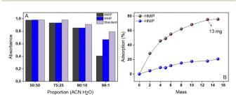
Fig. 4 Optimization of parameters that influence the DSPE analytical procedure. (A) optimization of solvent proportion; (B) optimization of HMIP and HNIP mass. n = 3
