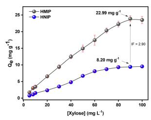
Fig. 6 Adsorption isotherm of xylose onto the HMIP and HNIP using a concentration range of 5 to 100 mg L<sup>-1</sup>. The HMIP exhibits a significantly higher adsorption capacity compared to the HNIP, confirming the presence of selective binding sites.
