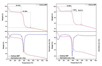
Fig. 3 TGA analysis of HMIP and HNIP: hollow-MIP (red line) and derivative (blue line).
