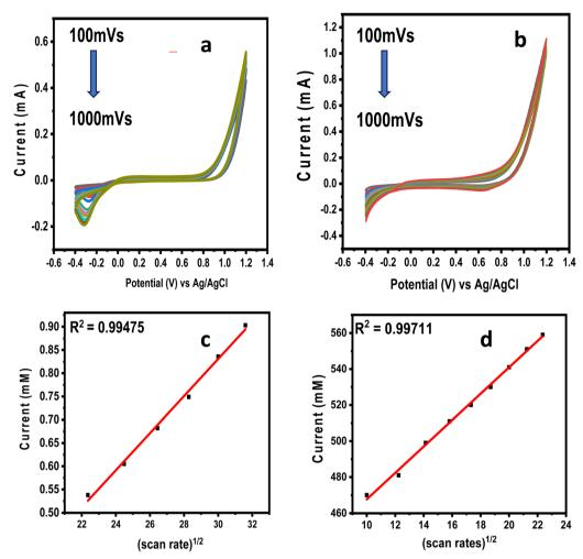
Fig. 7 Cyclic voltammogram of (a) CuMn-LDHs, (b) CuMn-LDHs/r-GO modified AuE recorded in 0.05 M NaOH at varied scan rates (100-1000 mV s<sup>-1</sup>), (c) and (d) the linear regression curves for (c) CuMn-LDHs and (d) CuMn-LDHs/r-GO modified AuE as a plot between the square root of scan rate and anodic peak current.
