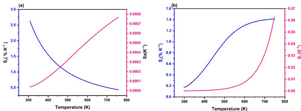
Fig. 9 Calculated absolute sensitivity ( $S_a$ ) and relative sensitivity ( $S_r$ ) of LiCaLa(MoO<sub>4</sub>)<sub>3</sub>:Tm<sup>3+</sup>/Yb<sup>3+</sup> phosphors in the temperature range 298–748 K, based on: (a) thermally coupled levels (TCL) using the emission intensity ratio at 700 nm and 800 nm. (b) Non-thermally coupled levels (NTCL) using the emission intensity ratio at 700 nm and 475 nm.
