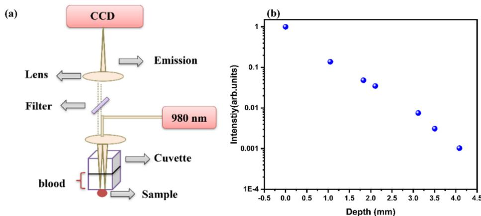
Fig. 13 (a) Experimental procedures for determining the depth of penetration (b) luminescence intensity as a function of the depth of the blood as obtained for the emission of 800 nm of LCLMO doped  $\text{Tm}^{3+}/\text{Yb}^{3+}$  with 975 nm excitation.
