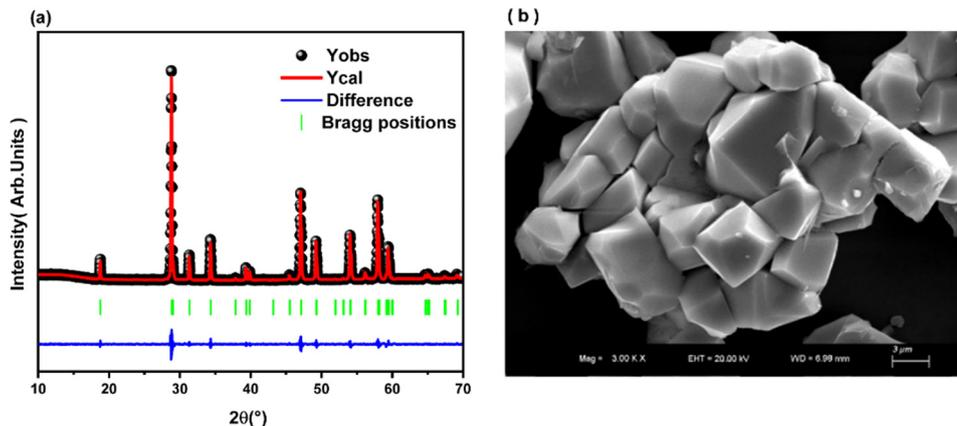
Fig. 2 (a) Rietveld refinement of the XRD pattern with  $\chi^2 = 1.32$  and  $R_{wp} = 9.63$ , (b) SEM image of LiCaLa(MoO<sub>4</sub>)<sub>3</sub>:Tm<sup>3+</sup>/Yb<sup>3+</sup> particles showing the surface morphology.
