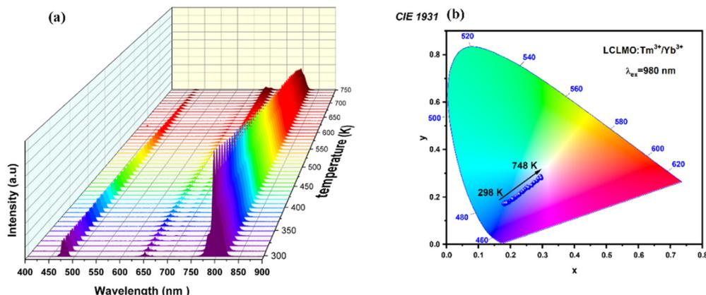
Fig. 7 (a) Temperature-dependent upconversion emission spectra of  $\text{LiCaLa}(\text{MoO}_4)_3:\text{Tm}^{3+}/\text{Yb}^{3+}$  phosphors recorded in the range 298 K to 748 K under 975 nm excitation. (b) Corresponding CIE chromaticity diagram showing the variation of emission color with temperature.
