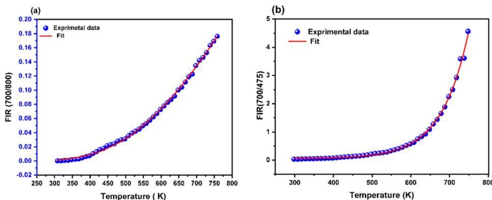
Fig. 8 Experimental fluorescence intensity ratio (FIR) as a function of temperature (298–748 K) for LiCaLa(MoO<sub>4</sub>)<sub>3</sub>:Tm<sup>3+</sup>/Yb<sup>3+</sup> phosphors: (a) FIR based on thermally coupled levels (TCL) at 700 nm and 800 nm. (b) FIR based on non-thermally coupled levels (NTCL) at 700 nm and 475 nm.
