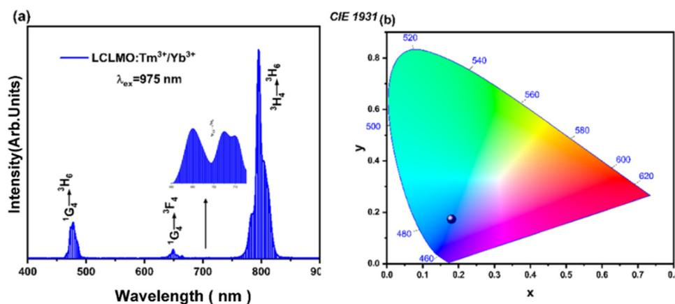
Fig. 4 (a) Upconversion emission spectra of  $\text{LiCaLa}(\text{MoO}_4)_3:\text{Tm}^{3+}/\text{Yb}^{3+}$  phosphors under 975 nm excitation. (b) Corresponding CIE 1931 chromaticity diagram showing the emission color coordinates of the doped sample.
