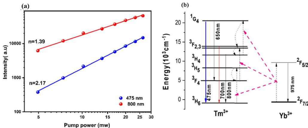
Fig. 6 (a) Upconversion emission intensity of  $\text{LiCaLa}(\text{MoO}_4)_3:\text{Tm}^{3+}/\text{Yb}^{3+}$  phosphors as a function of pump power under 975 nm excitation. (b) Schematic energy level diagram of  $\text{Tm}^{3+}$  and  $\text{Yb}^{3+}$  ions illustrating the upconversion mechanism in the LCLMO host matrix.
