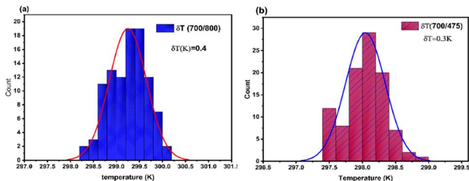
Fig. 11 Histograms of temperature distribution obtained from 100 repeated measurements (a) TCL 700/800 (b) NTCL 700/475, at room temperature of LCLMO doped  $\text{Tm}^{3+}/\text{Yb}^{3+}$  at room temperature.
