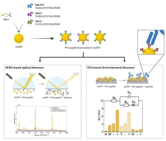
Fig. 1 Schematic representation of the optical and electrochemical biosensor operation. AuNPs were functionalized with the immunodominant P44 peptide in phosphate buffer (pH 6.0) using MBA as a Raman reporter. The biosensor detects antibodies in serum samples from convalescent COVID-19 patients and healthy individuals through Raman-SERS analysis combined with PLS-DA classification and electrochemical impedance measurements.
