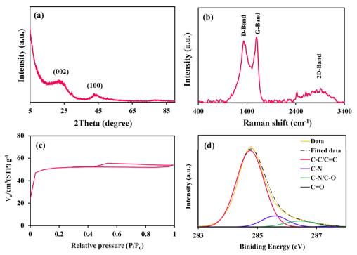
(a) XRD pattern, (b) Raman spectrum, (c) BET diagram, and (d) XPS curve of the CF.
