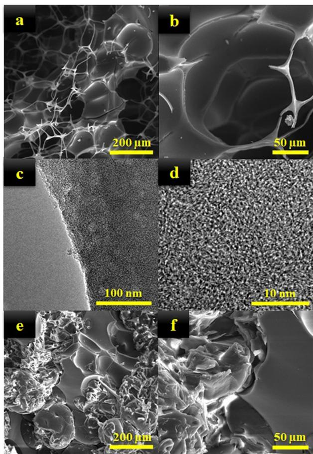
Fig. 2 (a) and (b) SEM images of the obtained CF at different magnifications, (c) and (d) TEM images of the porous structure of the synthesized CF, and (e) and (f) SEM images of the encapsulation of PCMs in the porous structure of the CF.
