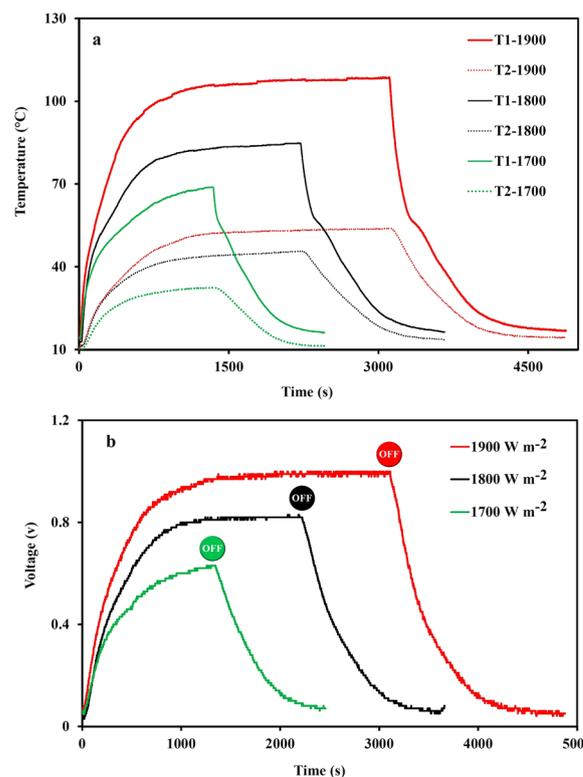
Fig. 7 (a) Temperature–time curves, and (b) open-circuit voltage of the thermoelectric conversion system with the CF/PW composite under the light intensities of 1700, 1800 and 1900 W m<sup>-2</sup>, respectively.
