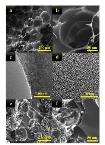
Fig. 2 (a) and (b) SEM images of the obtained CF at different magnifications, (c) and (d) TEM images of the porous structure of the synthesized CF, and (e) and (f) SEM images of the encapsulation of PCMs in the porous structure of the CF
