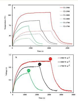
Fig. 7 (a) Temperature–time curves, and (b) open-circuit voltage of the thermoelectric conversion system with the CF/PW composite under the light intensities of 1700, 1800 and 1900 W  $m^{-2}$ , respectively.
