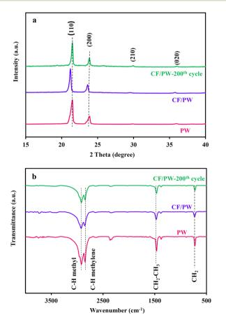
Fig. 4 (a) XRD patterns (b) FTIR spectra of PW and the CF/PW composite before and after thermal cycles.
